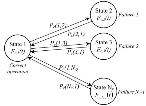
Fig. 2. Model for the generic component  $c$  of the power system.
