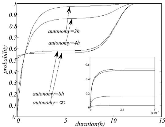
Fig. 6. Effect of the autonomy on the outage duration distribution.
