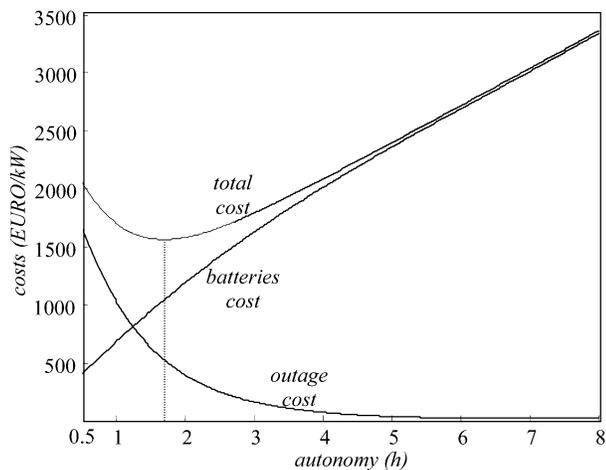
Fig. 7. Optimization of the storage autonomy minimizing the total cost.
