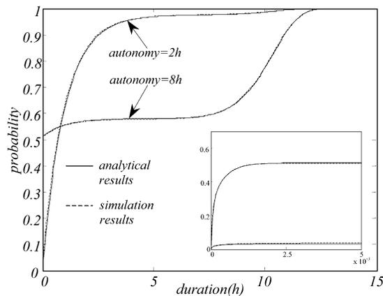
Fig. 5. Comparison between the analytical and simulation results for the outage duration distributions.
