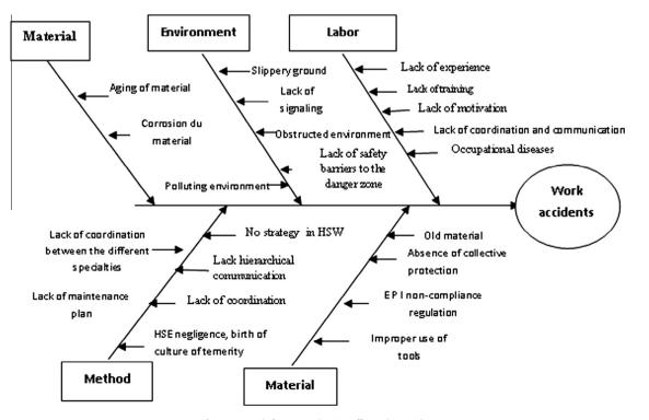
Fig. 11. Search for causes having effects the accident.
