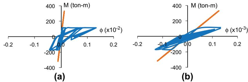
Fig. 8. Moment–curvature response of frame C-8N when subjected to two records with different predominant period: (a)  $T/T_g = 0.53$ , (b)  $T/T_g = 1.04$ .
