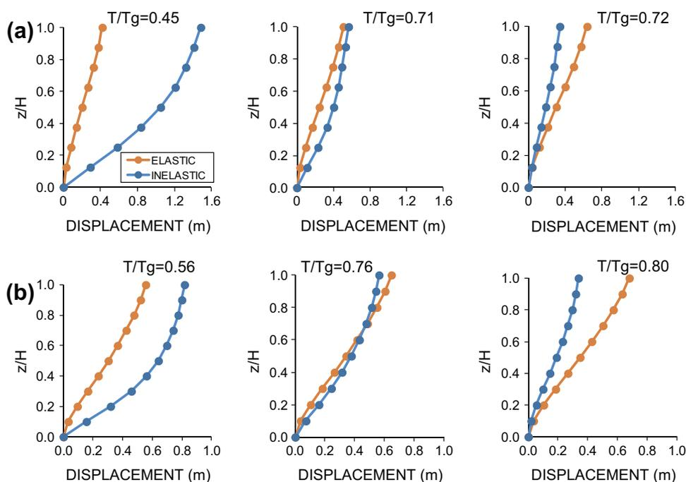
Fig. 5. Lateral displacement profiles computed for steel frames subjected to three records with different predominant period: (a) frame A-8N, (b) frame A-10N.
