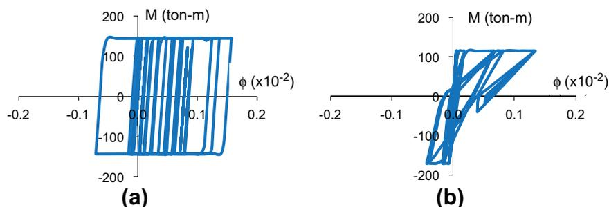
Fig. 3. Element hysteretic behavior considered in this study: (a) quasi-elastoplastic model (steel frames), (b) Takeda model (RC frames).
