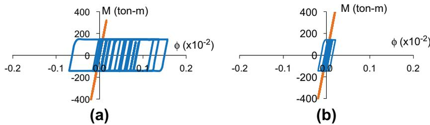
Fig. 7. Moment–curvature response of frame A-10N when subjected to two records with different predominant period: (a)  $T/T_g = 0.40$ , (b)  $T/T_g = 0.83$ .
