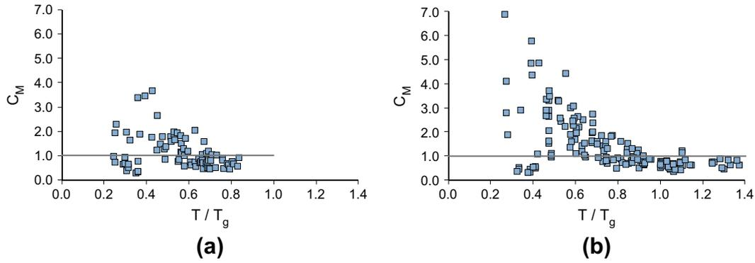
Fig. 12. Ratio of the inelastic displacement ratio computed from MDOF systems: (a) steel frames, (b) RC frames.
