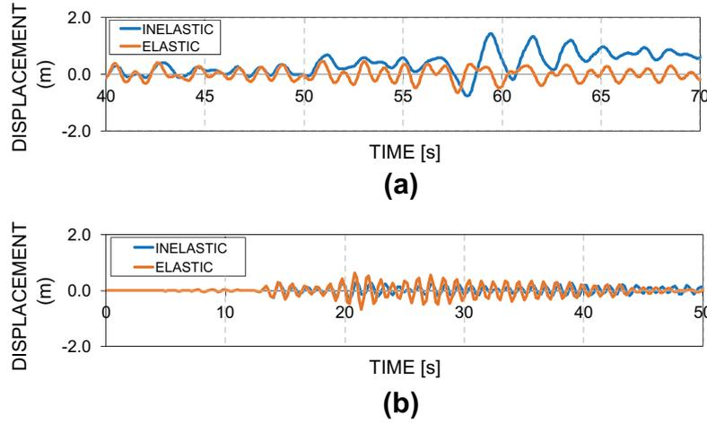
Fig. 9. Roof displacement time–history response of frame A-10N when subjected to two records with different predominant period: (a)  $T/T_g = 0.40$ , (b)  $T/T_g = 0.83$ .
