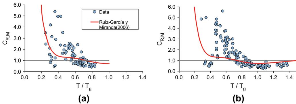
Fig. 11. Comparison of inelastic displacement ratios computed from the MDOF systems under consideration and predicted inelastic displacement ratio using Eq. (4): (a) steel frames, (b) RC frames.
