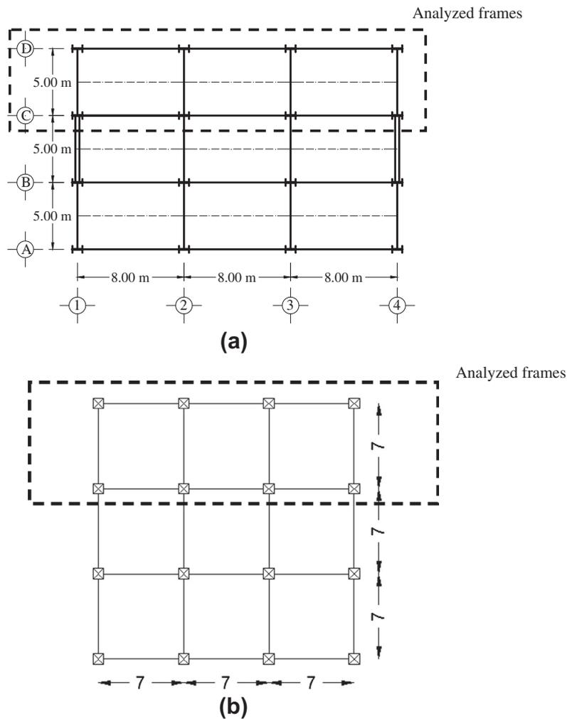
Fig. 2. Plan view of case-study buildings (units in meters): (a) steel buildings, (b) RC buildings.
