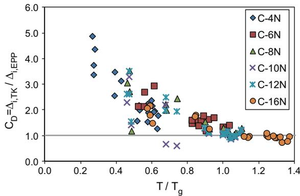
Fig. 13. Spectral distribution of ratios of maximum inelastic roof displacement demand taking into account member's Takeda-type hysteretic behavior to maximum inelastic roof displacement demand (denoted as  $C_D$ ) taking into account member's elastoplastic hysteretic behavior.
