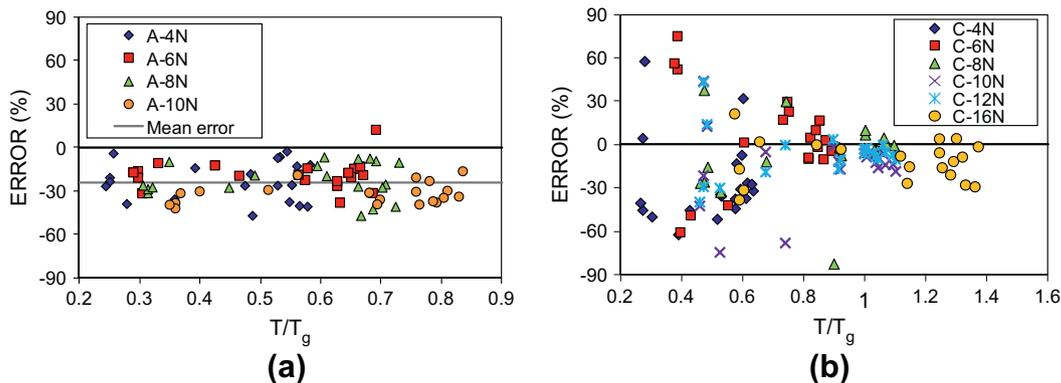
Fig. 17. Relative error of the Displacement Coefficient method to estimate maximum roof displacement demands; (a) steel frames, (b) RC frames.
