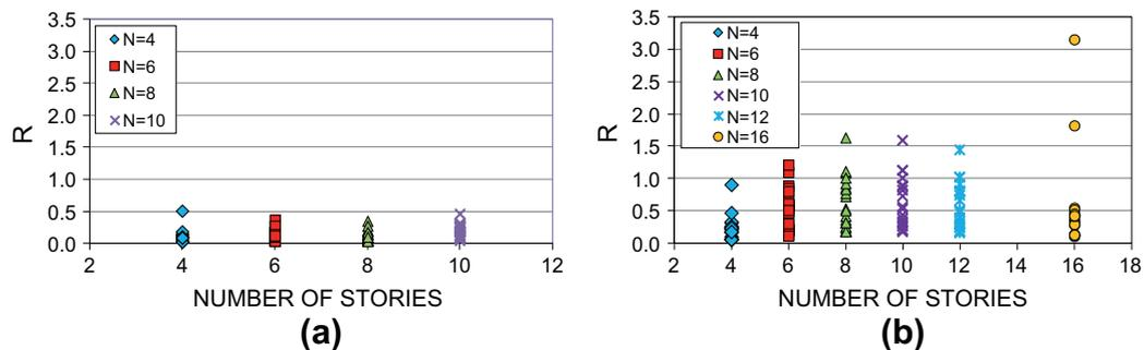
**Fig. 4.** Initial relative lateral strength ratio (i.e. from as-recorded earthquake ground motions) for the set of frames considered in this study: (a) steel frames, (b) RC frames.
