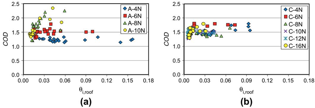
Fig. 15. Coefficient of distortion as a function of maximum roof drift: (a) steel frames, (b) RC frames.
