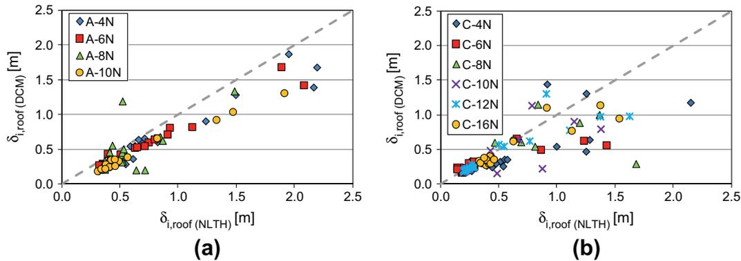
Fig. 16. Comparison of peak roof displacements computed from nonlinear time-history (NLTH) analyses with those computed with Displacement-Coefficient method: (a) steel frames, (b) RC frames.
