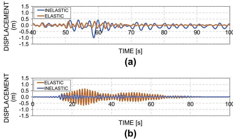
Fig. 10. Roof displacement time–history response of frame C-8N when subjected to two records with different predominant period: (a)  $T/T_g = 0.53$ , (b)  $T/T_g = 1.04$ .
