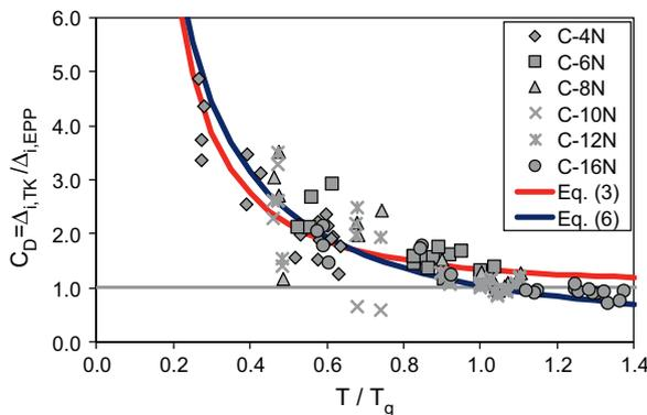
Fig. 14. Comparison of empirical  $C_D$  ratios with those computed from fitted Eqs. (3) and (6).
