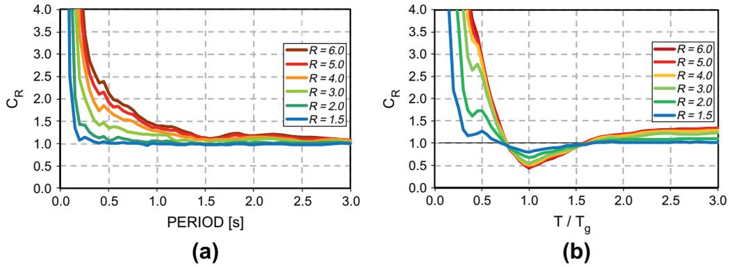
Fig. 1. Mean inelastic displacement ratio (i.e. coefficient  $C_1$ ) computed for: (a) firm soil sites (adapted from: [19]), (b) soft soil sites (adapted from: [20]).
