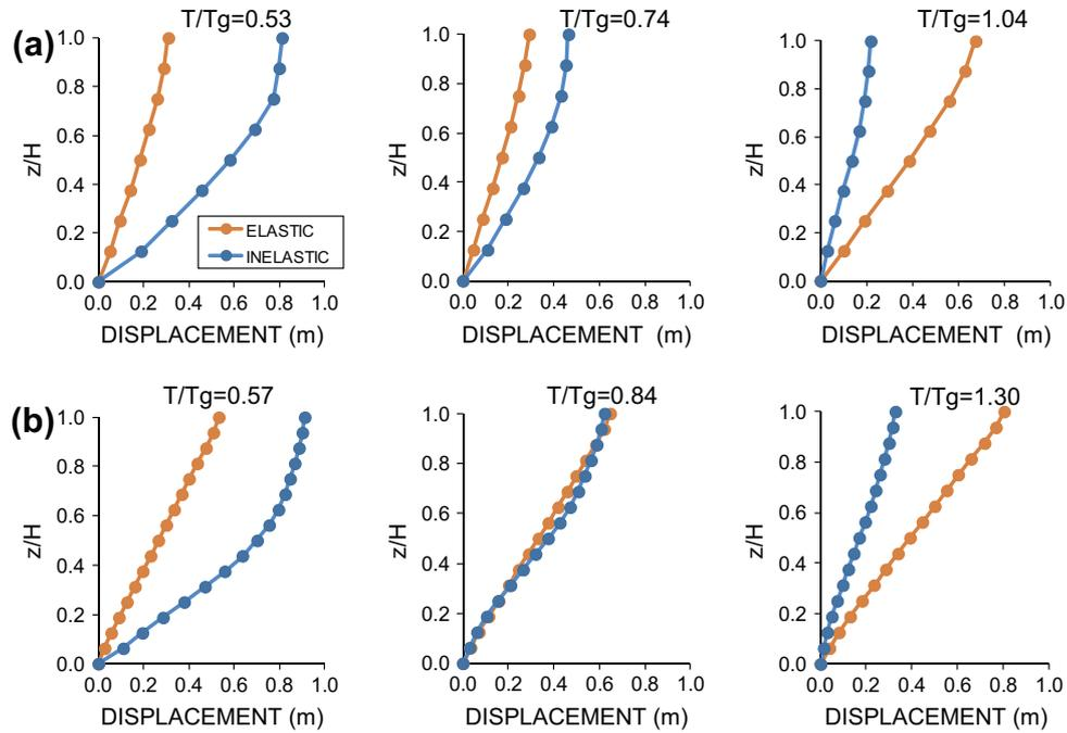
Fig. 6. Lateral displacement profiles computed for two RC frames subjected to three records with different predominant period: (a) frame C-8N, (b) frame C-16N.
