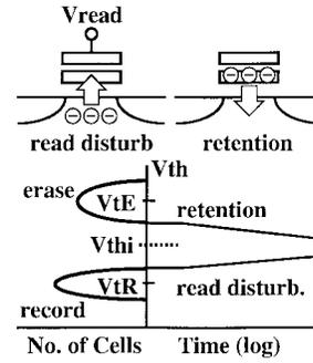
Fig. 13. Read disturbance and retention.
