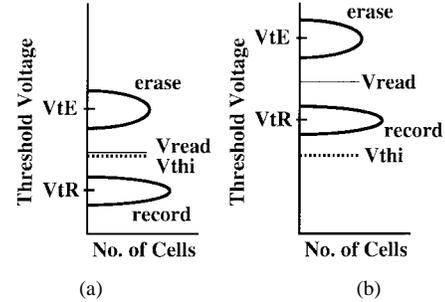
Fig. 14. Voltage relation of conventional and proposed asymmetrical schemes: (a) conventional and (b) proposed asymmetrical.
