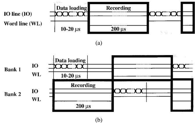
Fig. 9. Parallel recording and data loading: (a) serial operation and (b) parallel operation.
