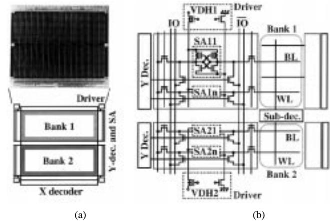
Fig. 8. Multibank Flash memory for continuous recording: (a) multibank chip and (b) circuit schematic.
