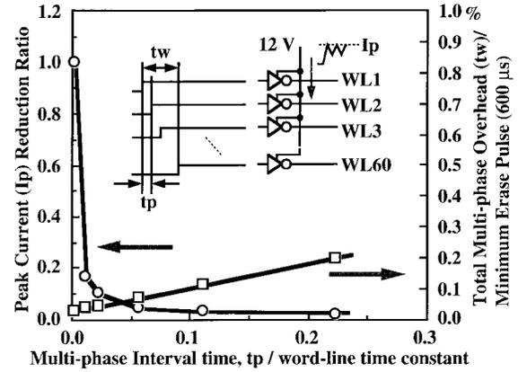
Fig. 11. Peak current in multiphase word driving.
