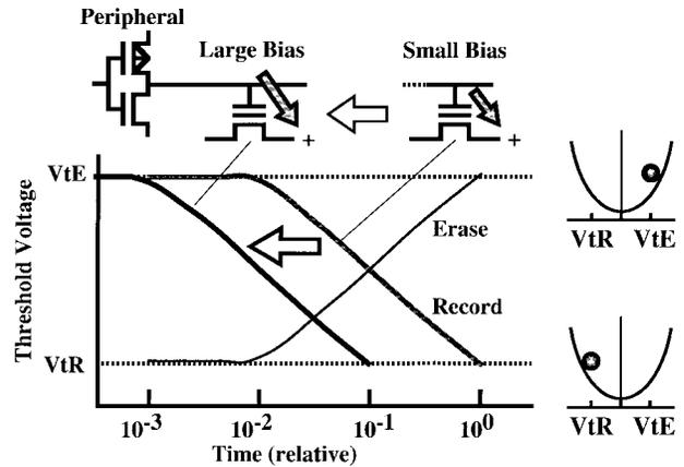
Fig. 3. Fast recording in conventional method.
