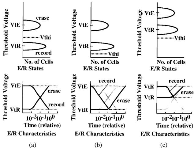
Fig. 5. Schematic cell threshold voltage distribution and erase/record (E/R) characteristics: (a) conventional, (b) proposed 1, and (c) proposed 2.
