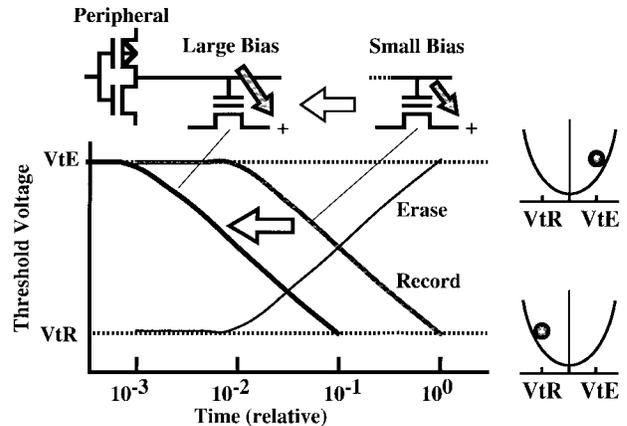
Fig. 3. Fast recording in conventional method.
