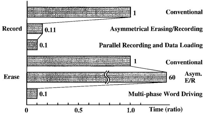
Fig. 12. Effect of high-speed erasing and recording.
