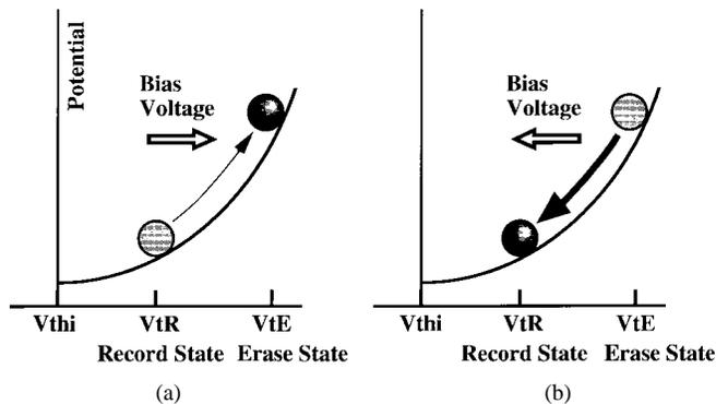
Fig. 4. Proposed asymmetrical operation: (a) erasing and (b) recording.
