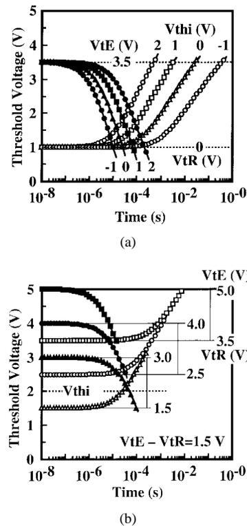
Fig. 6. Simulated asymmetrical characteristics: (a) erase/record characteristics versus  $V_{thi}$  and (b) erase/record characteristics versus  $V_{tE}$ ,  $V_{tR}$ .
