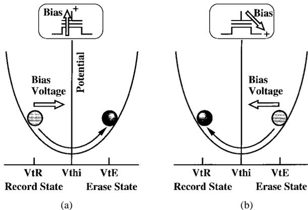
Fig. 2. Conventional symmetrical operation: (a) erasing and (b) recording.
