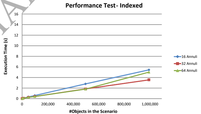
Figure 14: Performance and influence of the number of annuli in our approach using a PR-tree based indexing.
