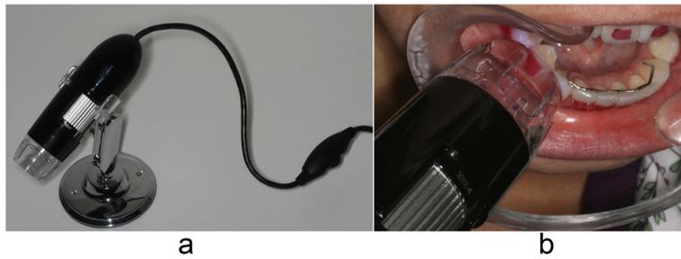
**Fig. 2** **a** Portable digital microscope used to determine the ARI. **b** Microscope being used
