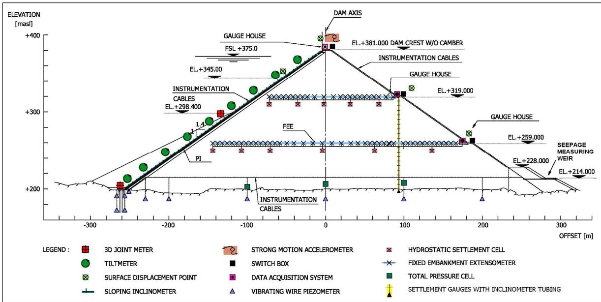
Figure 7: Arrangement of instruments at the riverbed section
