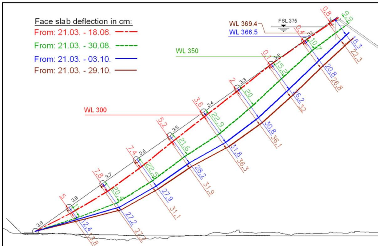
Figure 12: Face slab deflection derived from tiltmeter readings
