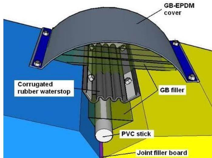
Figure 5: Schematic of GB<sup>®</sup>-Waterstop System
