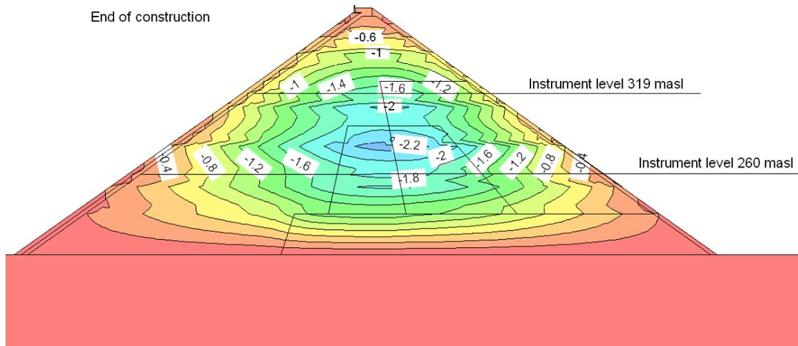
Figure 9: Dam settlements (in m) at the end of construction
