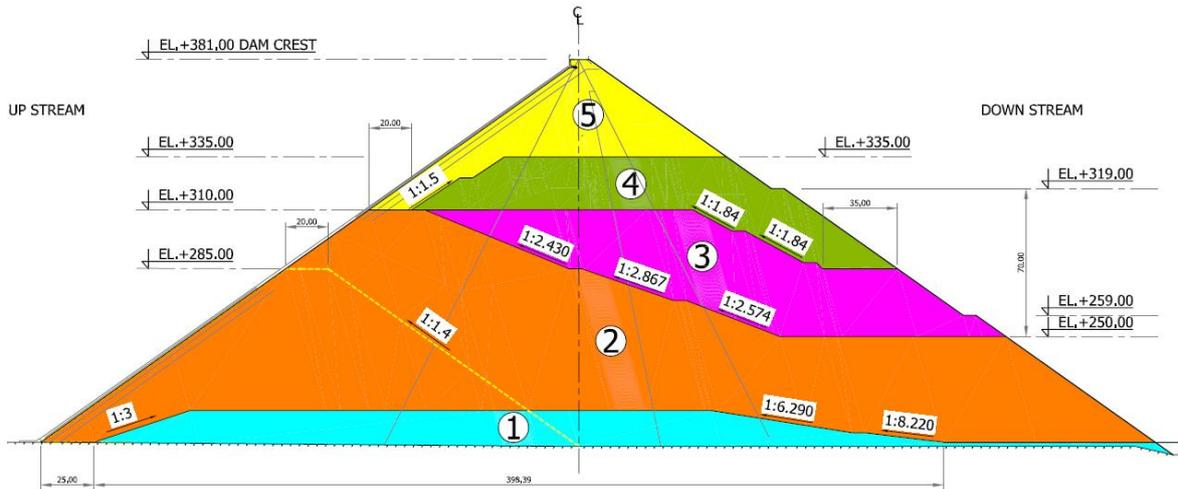
Figure 3: Stages of construction
