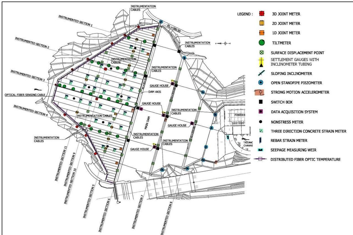
Figure 8: Overview of provided dam instrumentation
