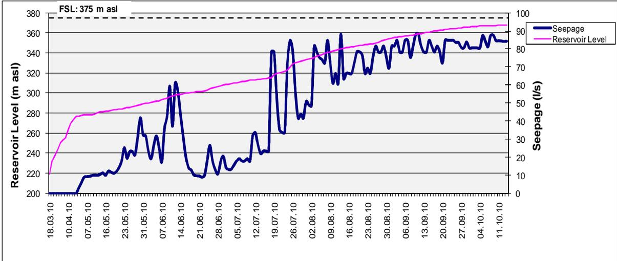
Figure 10: Seepage quantities and reservoir fill curve
