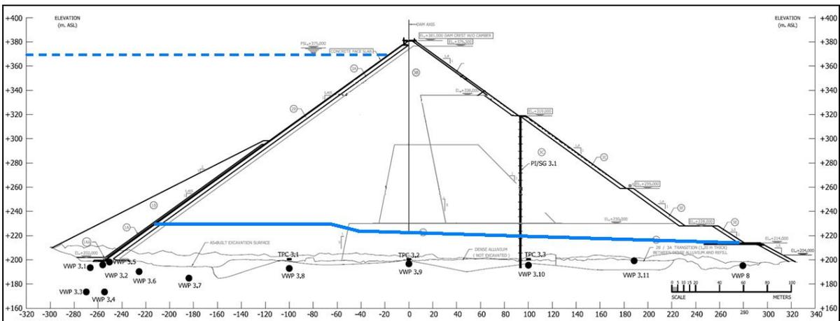
Figure 11: Water table in the dam body
