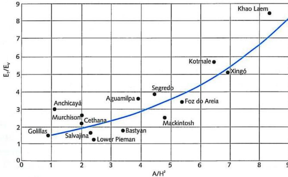
Figure 13: Ratio  $E_T/E_V$  as a function of  $A/H^2$  [2]
