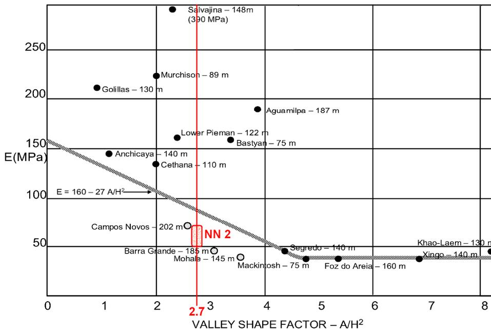
Figure 4: Graph deformation modulus vs. valley shape factor (after Pinto [1])
