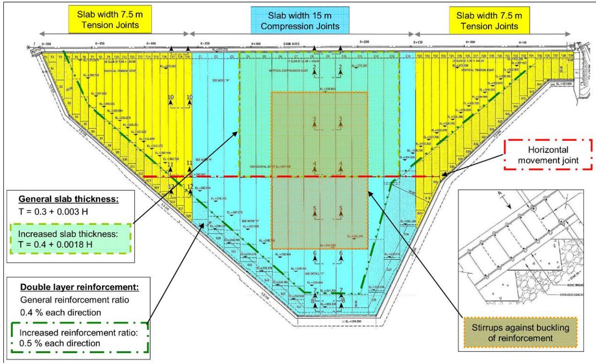
Figure 6: Face slab – main design features
