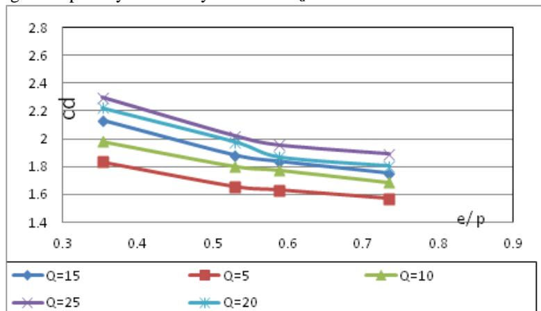
**Fig. 7:** Relation of effect of spillway relative roughness than discharge coefficient.
