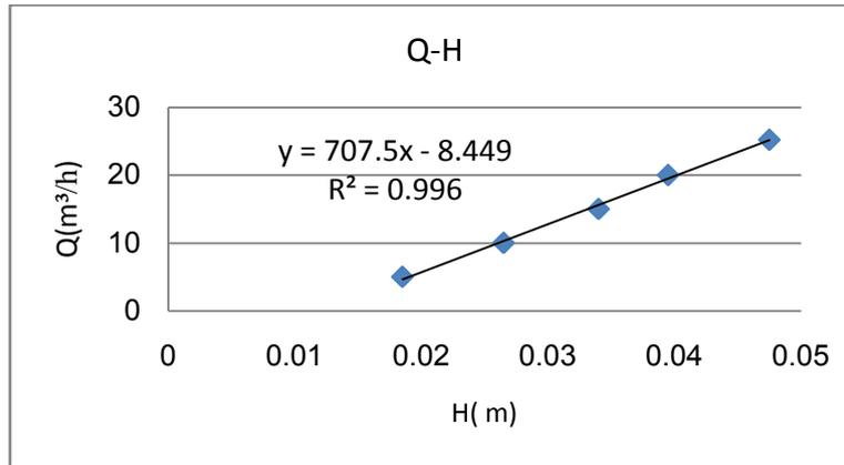
**Fig. 6:** Relation of scale flow rate for spillway with flat bed.
