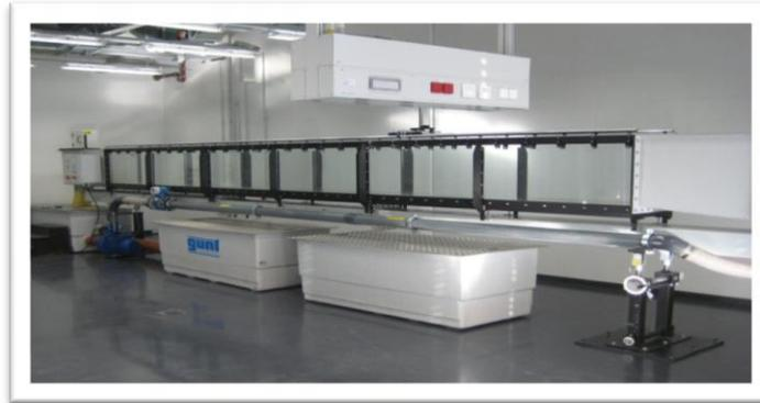
**Fig. 2:** 7.5 m flume which is set up and implemented in laboratory.
