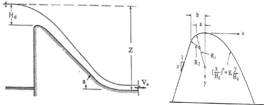
**Fig. 1:** Ogee spillway.
