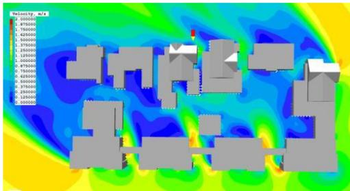
Fig. 5. wind speed levels – corridor on F2 enclosed.
