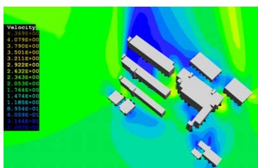
Fig. 8. summertime wind speed levels –teaching building 31-34 with partial open-up design.
