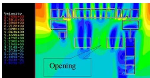
Fig. 10. summertime wind speed levels –teaching building 31 with opening in building shape.
