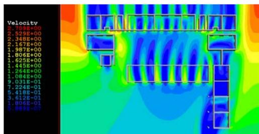
Fig. 9. summertime wind speed levels –teaching building 31 with no opening in building shape.
