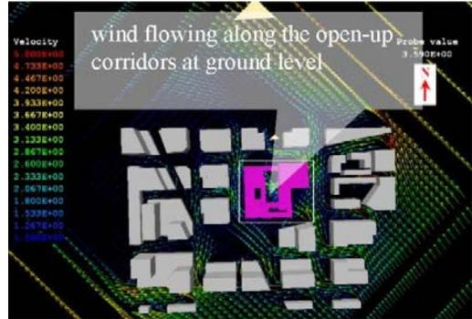
Fig. 2. vector of wind speed distribution at pedestrian height around the building.
