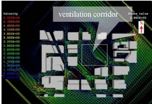
Fig. 1. vector of wind speed distribution at pedestrian height on the site.
