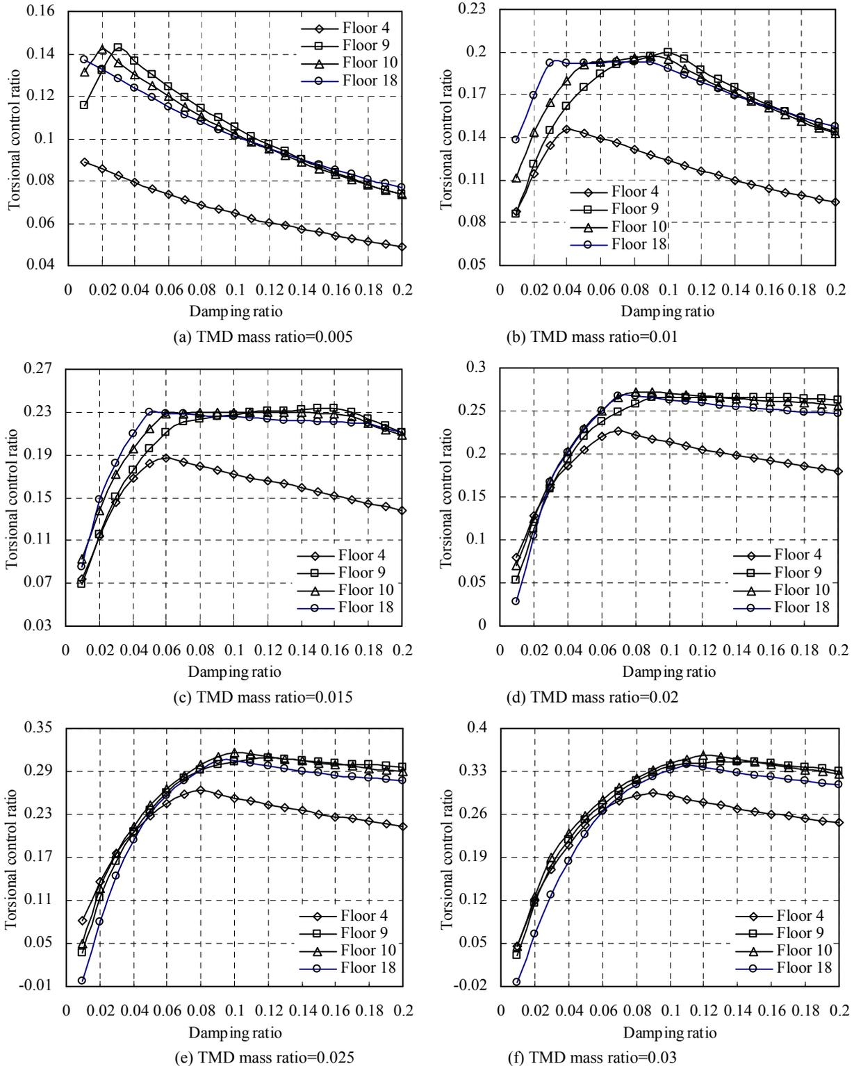
Fig. 2 Relationship between torsional control ratio and damping ratio
