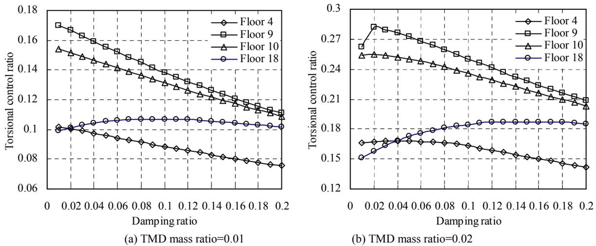
Fig. 3 Relationship between torsional control ratio and damping ratio
