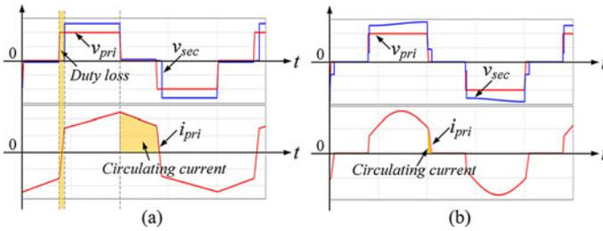
Fig. 11. Comparative analysis of duty loss and circulating currents: (a) conventional PSFB converter and (b) proposed HSPSFB dc-dc converter.
