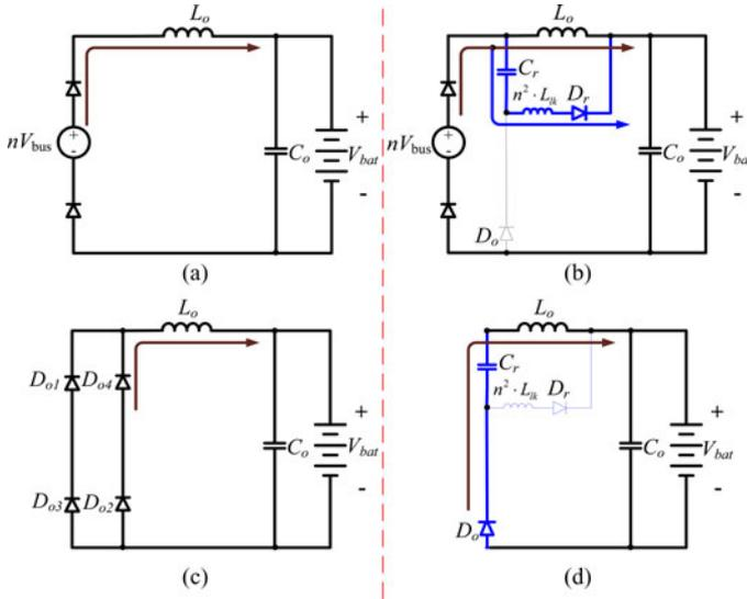
Fig. 10. Steady-state secondary-side equivalent circuits of traditional PSFB dc-dc converter and the proposed HSPSFB dc-dc converter. (a) Active stage of traditional PSFB dc-dc converter. (b) Active stage of proposed HSPSFB dc-dc converter. (c) Freewheeling stage of traditional PSFB dc-dc converter. (d) Freewheeling stage of proposed HSPSFB dc-dc converter.
