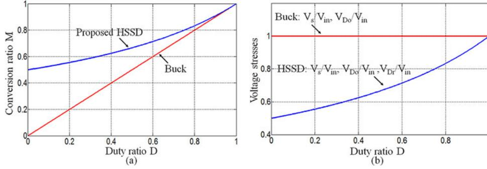
Fig. 4. (a) Voltage conversion ratios of the proposed HSSD and buck dc-dc converters. (b) Voltage stresses of devices of the proposed HSSD and buck dc-dc converters.
