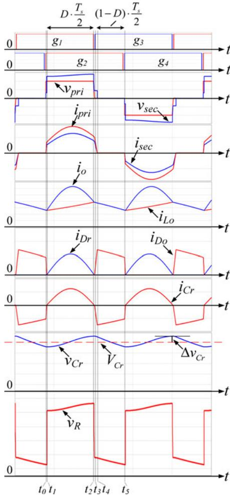
Fig. 7. Key waveforms of the proposed HSPSFB dc-dc converter in Mode 2 operation.
