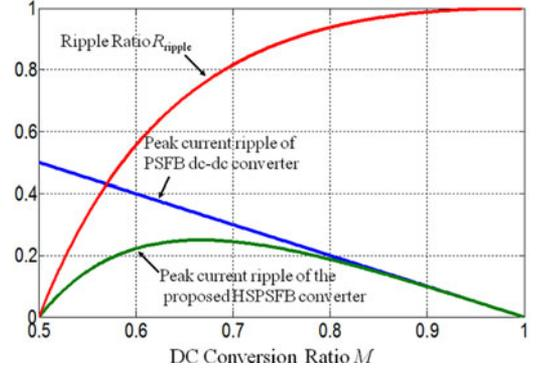
Fig. 13. Normalized peak current ripple of the traditional PSFB dc-dc converter, the proposed HSPSFB dc-dc converter, and current ripple ratio of proposed converter to traditional PSFB converters.
