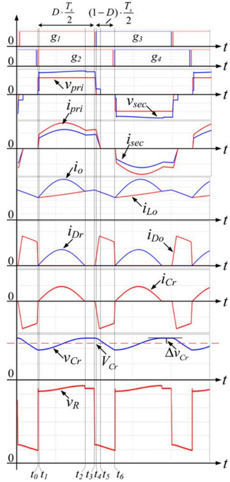
Fig. 6. Key waveforms of the proposed HSPSFB dc-dc converter in Mode 1 operation.
