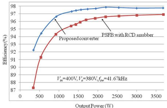
Fig. 18. Efficiency curves for proposed converter and traditional PSFB dc-dc converter with RCD snubber.
