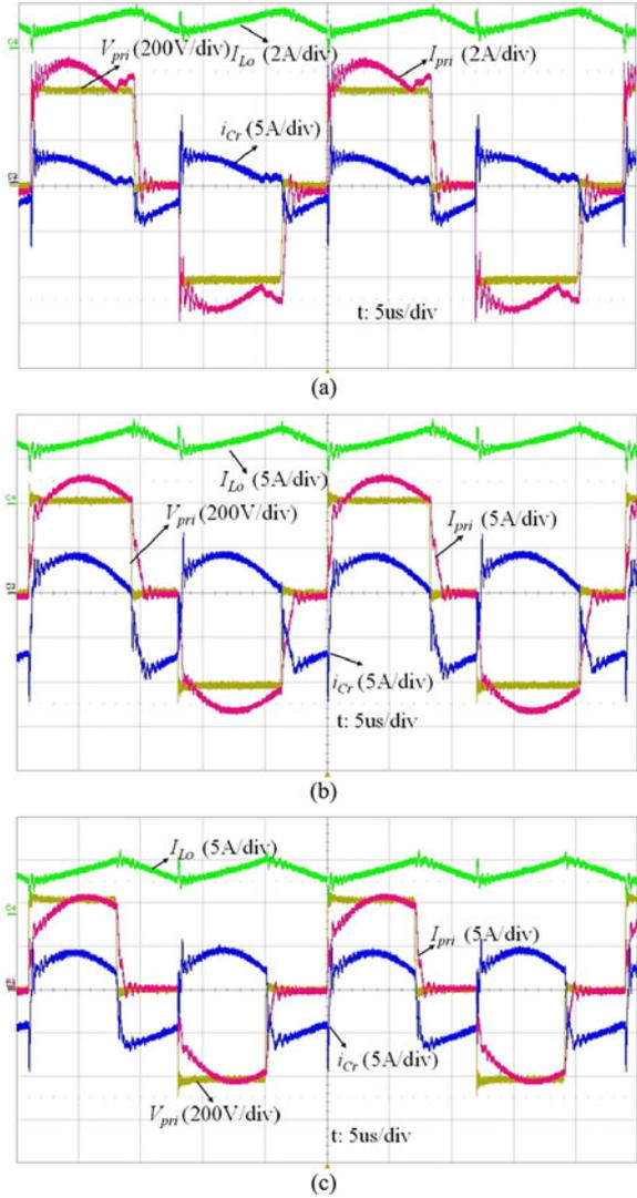
Fig. 14. Experimental waveforms for three different operation modes: (a) Mode 1:  $V_{in} = 400$  V,  $V_o = 360$  V,  $P_o = 1.3$  kW; (b) Mode 2:  $V_{in} = 400$  V,  $V_o = 330$  V,  $P_o = 3.1$  kW; and (c) Mode 3:  $V_{in} = 400$  V,  $V_o = 300$  V,  $P_o = 2.2$  kW.
