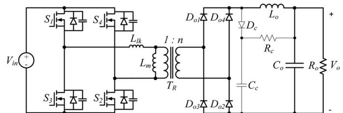
Fig. 1. Conventional PSFB dc-dc converter with an RCD snubber.
