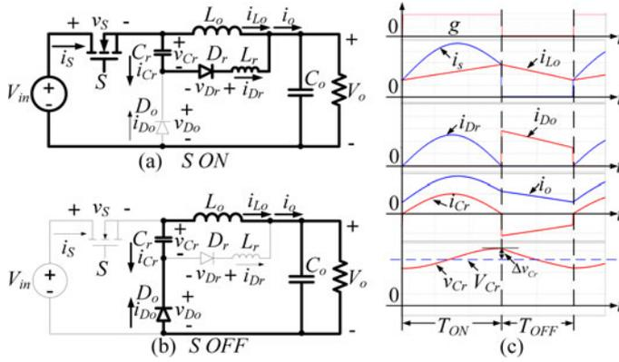
Fig. 3. (a) Topological stage during on-time interval, (b) topological stage during off-time interval, and (c) key waveforms.
