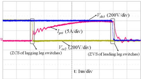
Fig. 16. ZVS for leading-leg switches and ZCS for lagging-leg switches.
