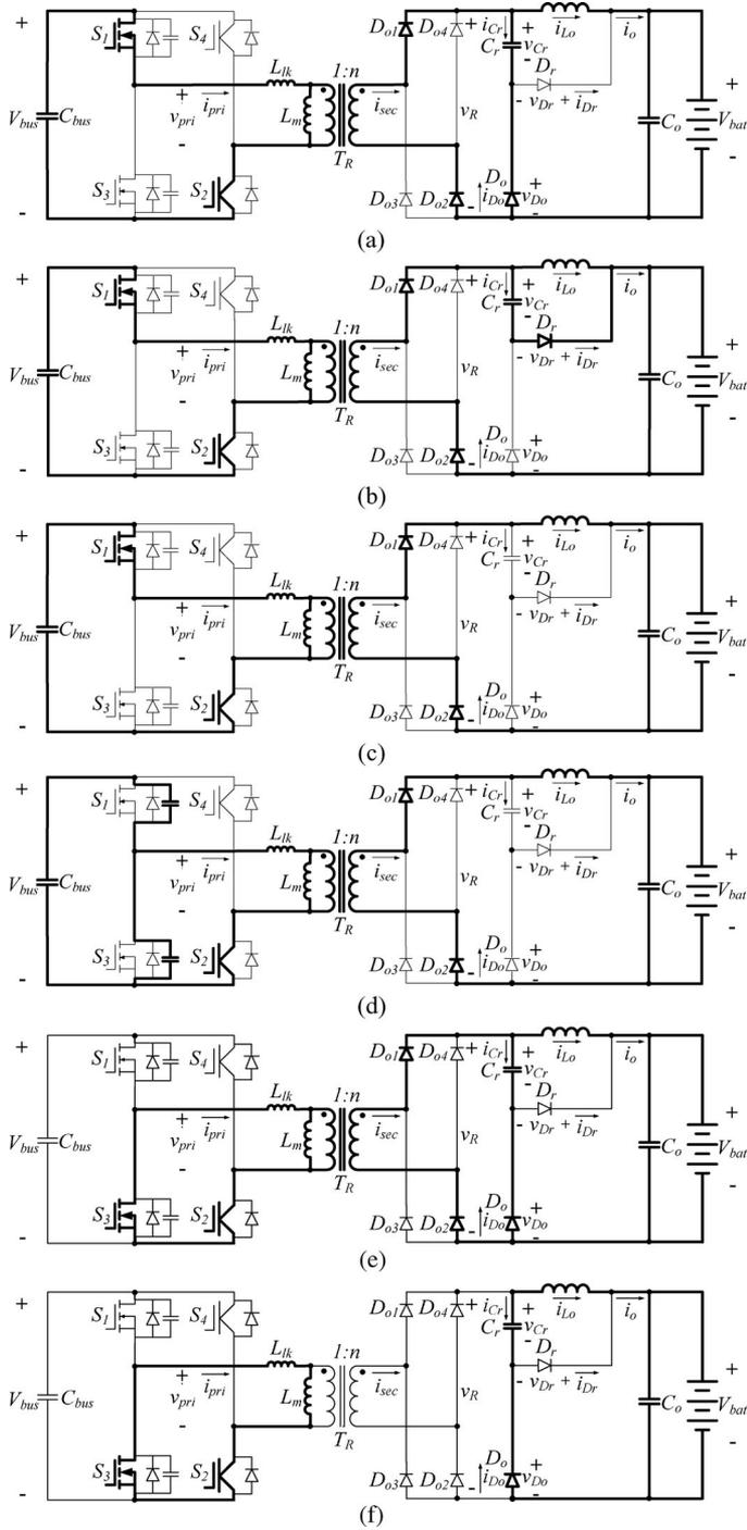
Fig. 5. Topological stages of the proposed HSPSFB dc-dc converter in Mode 1 operation. (a)  $[t_0, t_1]$ , (b)  $[t_1, t_2]$ , (c)  $[t_2, t_3]$ , (d)  $[t_3, t_4]$ , (e)  $[t_4, t_5]$ , and (f)  $[t_5, t_6]$ .
