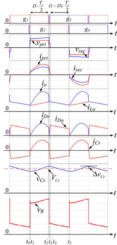
Fig. 8. Key waveforms of the proposed HSPSFB dc-dc converter in Mode 3 operation.
