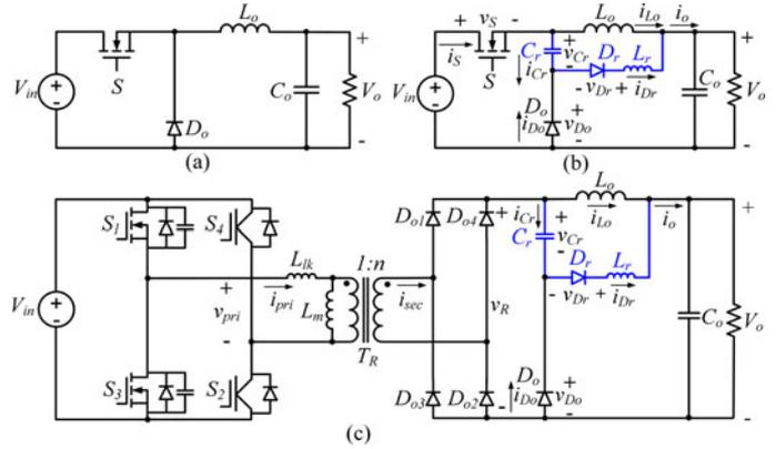
Fig. 2. (a) Conventional PWM buck dc–dc converter, (b) proposed hybrid-switching step-down dc–dc converter, (c) proposed ZVZCS hybrid-switching full-bridge dc–dc converter.
