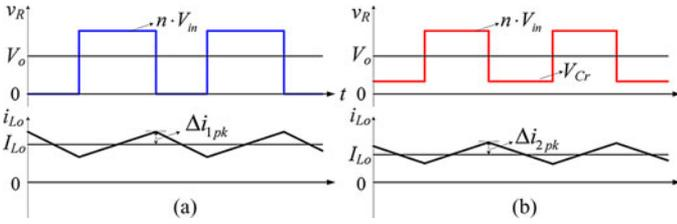
Fig. 12. Simplified rectified voltage waveforms of conventional PSFB converter and proposed HSPSFB dc-dc converter.
