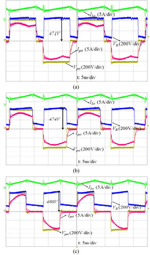
Fig. 15. Experimental waveforms demonstrating the secondary-side rectifier output voltage  $V_R$ : (a) Mode 1, (b) Mode 2, and (c) Mode 3 operations.
