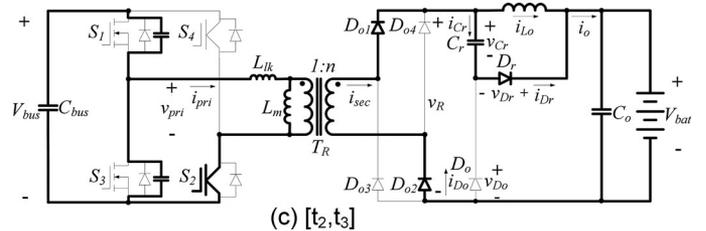
Fig. 9. Topological Stage 3 in Mode 3 operation.
