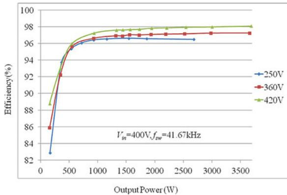
Fig. 17. Measured efficiencies.
