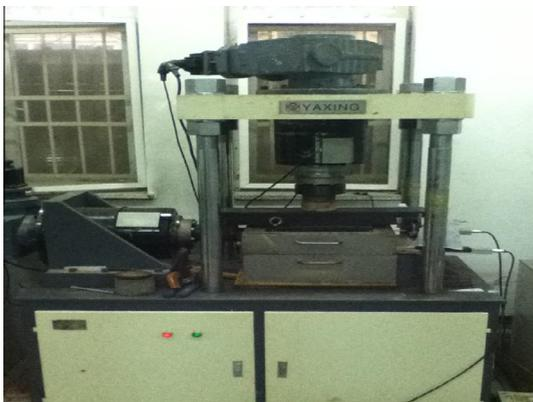
Fig. 2. Large-scale direct shear apparatus at Beijing Jiaotong University.
