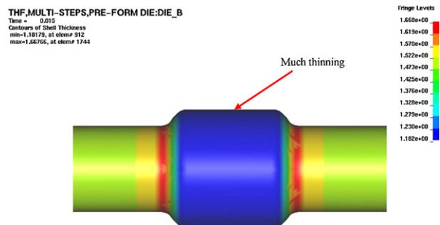
**Fig. 12 – Thickness distribution when using 7.0 MPa feeding pressure in the pre-forming stage.**
