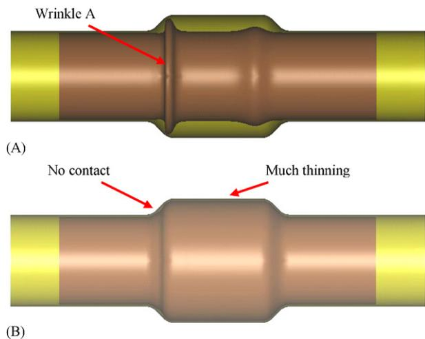
**Fig. 9 – Forming processes under 3.0 MPa feeding pressure in the pre-forming stage. (A) After feeding pressure; (B) after calibration pressure.**
