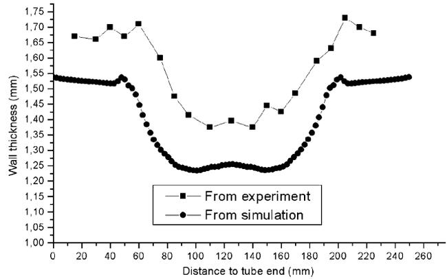
**Fig. 25 – Wall thickness distributions along axial direction profile between simulation and experiment after the pre-forming stage.**
