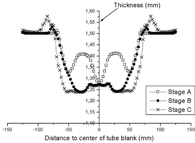
**Fig. 20 – Wall thickness distributions in different stages under feeding pressure of 5.0 MPa in the pre-forming stage.**
