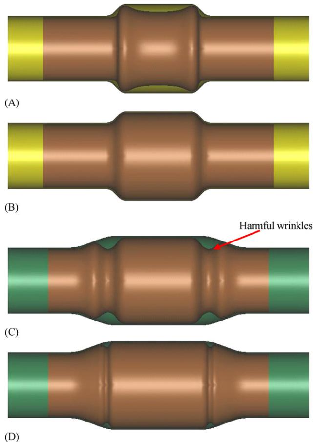
**Fig. 11 – Forming processes under 6.0 MPa feeding pressure in the pre-forming stage. (A) After feeding pressure in the pre-forming stage; (B) after calibration pressure in the pre-forming stage; (C) after feeding pressure in the finishing stage; (D) after calibration pressure in the finishing stage.**
