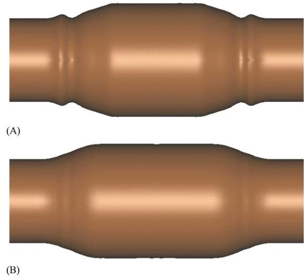
Fig. 17 – Final part by using very high calibration pressure 80.0 MPa in the finishing stage. (A) After feeding pressure; (B) after calibration pressure.
