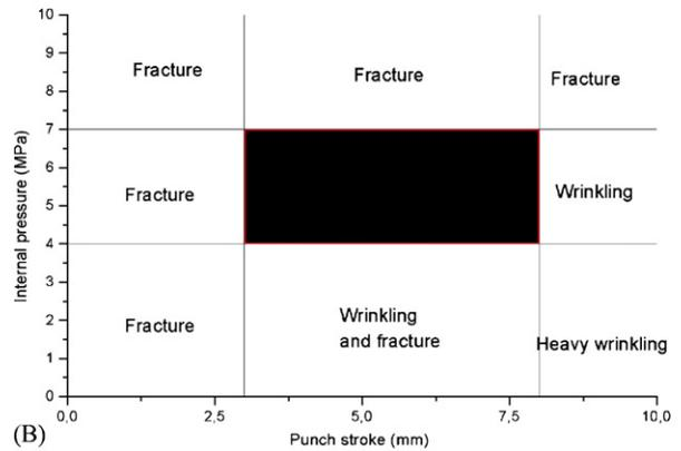
**Fig. 22 – Process windows for the feeding pressure and the punch stroke. (A) In the pre-forming stage; (B) in the finishing stage.**
