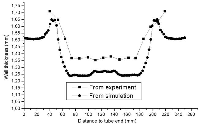
**Fig. 26 – Wall thickness distributions along axial direction profile between simulation and experiment after finishing stage.**
