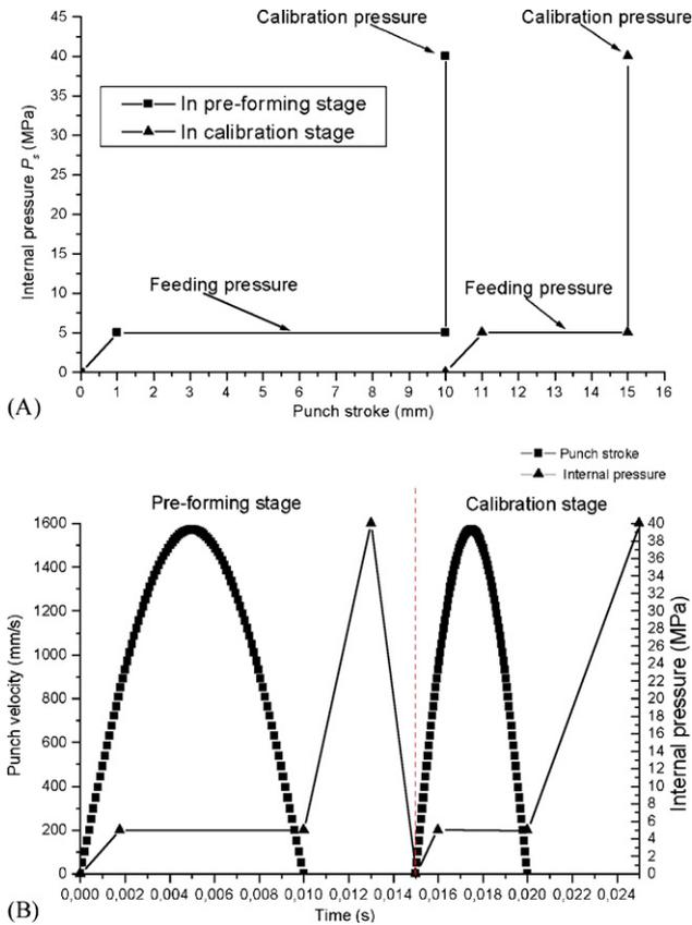
**Fig. 4 – Conceptual process parameters versus loading curves used in simulation. (A) Conceptual design for the process parameters; (B) practical usage in simulation.**
