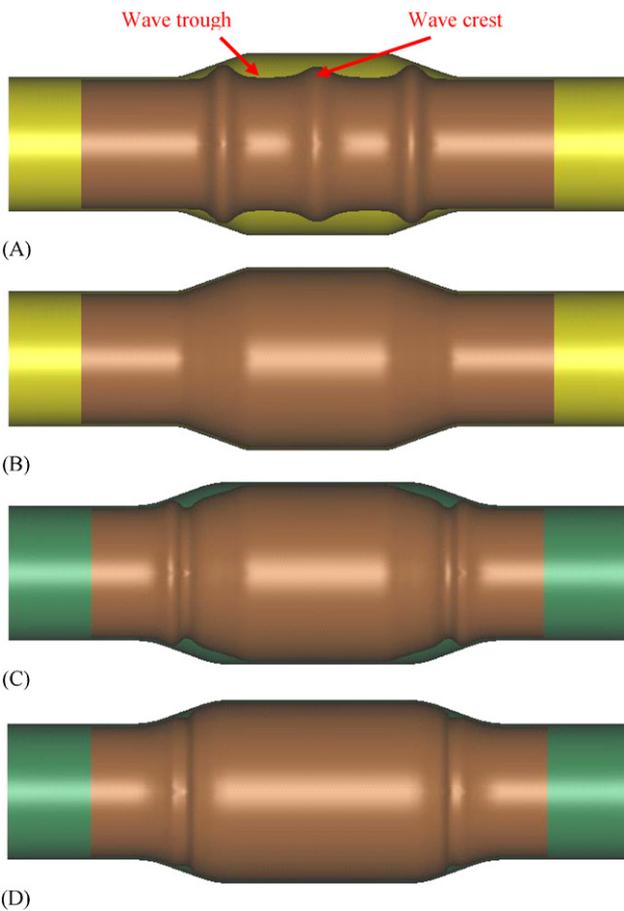
**Fig. 14 – Forming processes under 3.0 MPa internal pressure in the pre-forming stage. (A) After feeding pressure in the pre-forming stage; (B) after calibration pressure in the pre-forming stage; (C) after feeding pressure in the finishing stage; (D) after calibration pressure in the finishing stage.**
