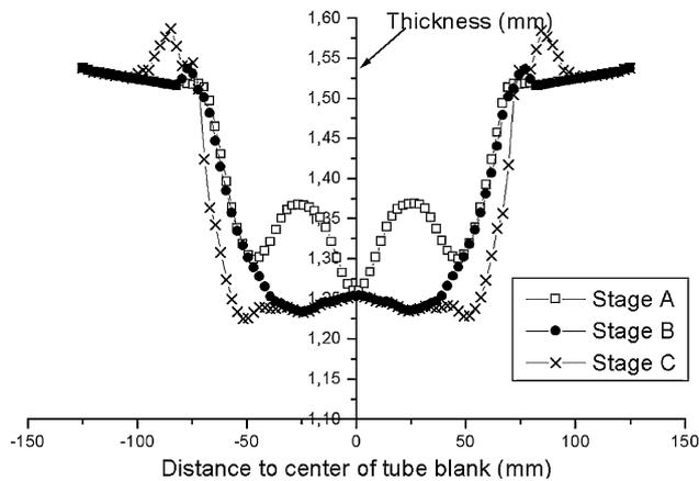
**Fig. 21 – Wall thickness distributions in different stages under feeding pressure of 6.0 MPa in the pre-forming stage.**
