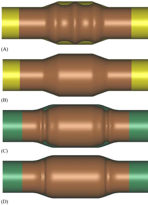
Fig. 16 – Forming processes under 6.0 MPa internal pressure in the pre-forming stage. (A) After feeding pressure in the pre-forming stage; (B) after calibration pressure in the pre-forming stage; (C) after feeding pressure in the finishing stage; (D) after calibration pressure in the finishing stage.
