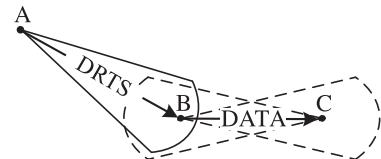
**Fig. 5.** Deafness due to directional antennas.
