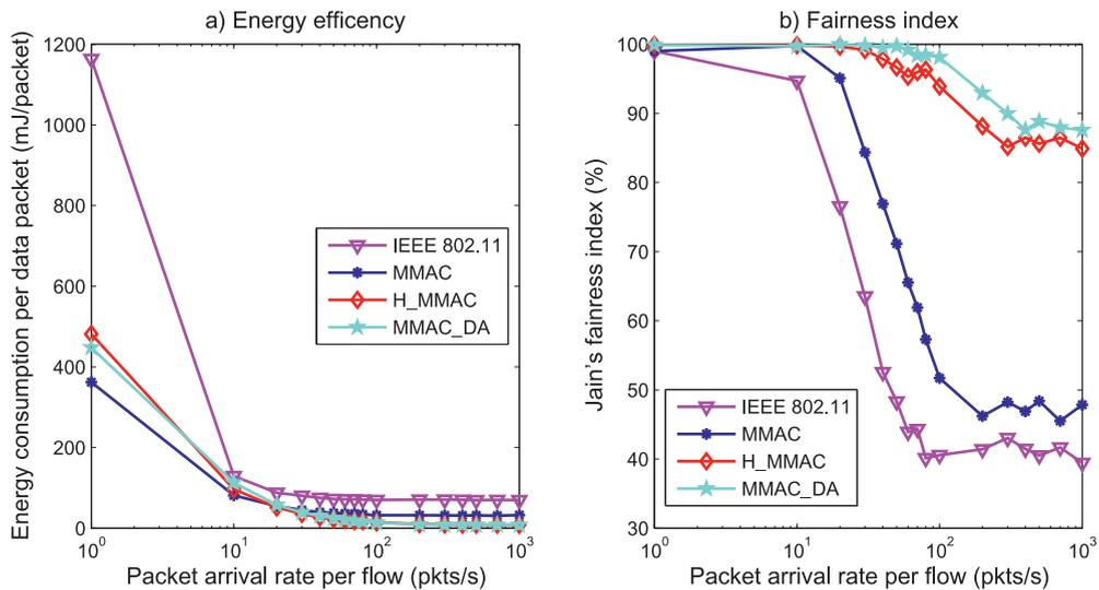
Fig. 16. Performance comparison of different protocols.
