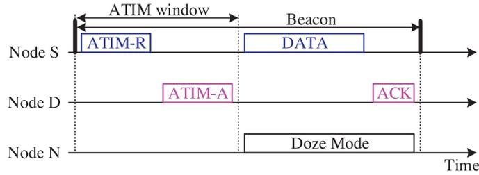
Fig. 7. The operation of IEEE 802.11 PSM.
