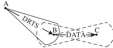
Fig. 5. Deafness due to directional antennas.
