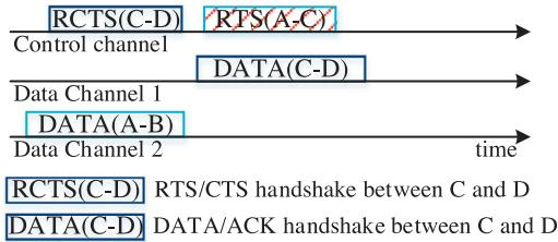
**Fig. 4.** Missing receiver due to multi-channel environment.
