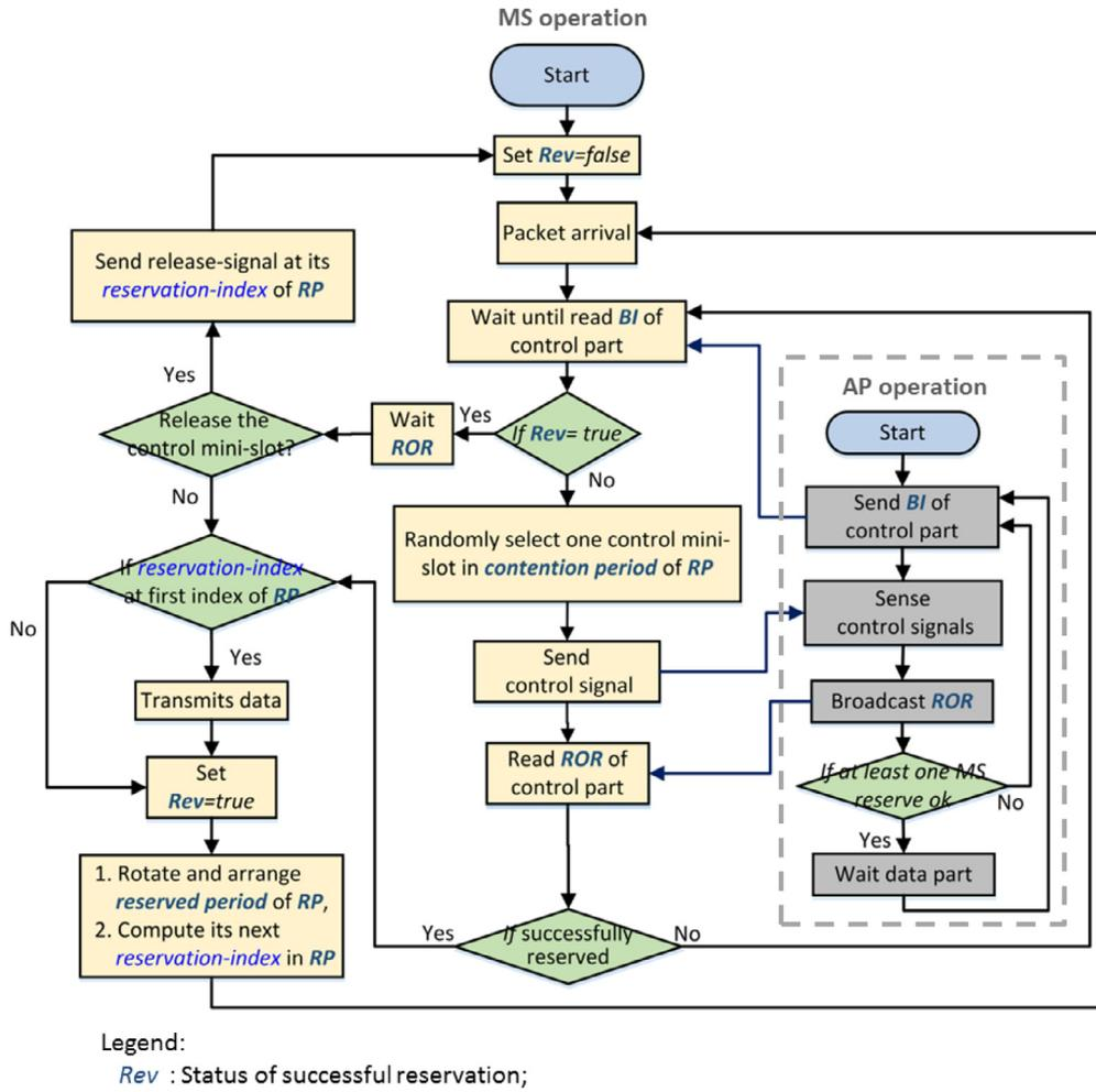
Fig. 2. The flow chart of the transmission procedure between AP and MSs.
