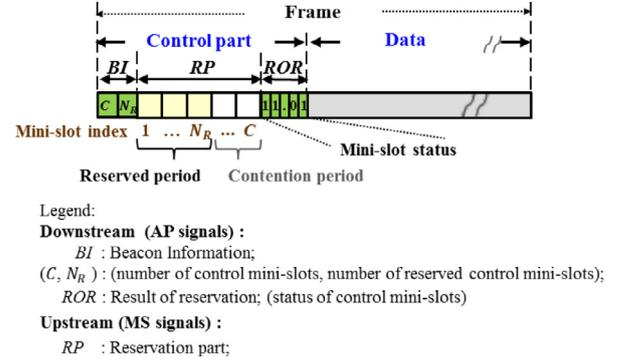
Fig. 1. The frame structure: control part and data.
