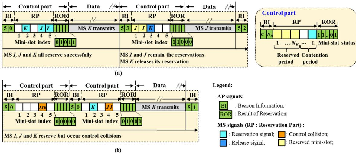
Fig. 3. Examples of the proposed MAC scheme. (a) Without control part collisions. (b) With control part collisions.
