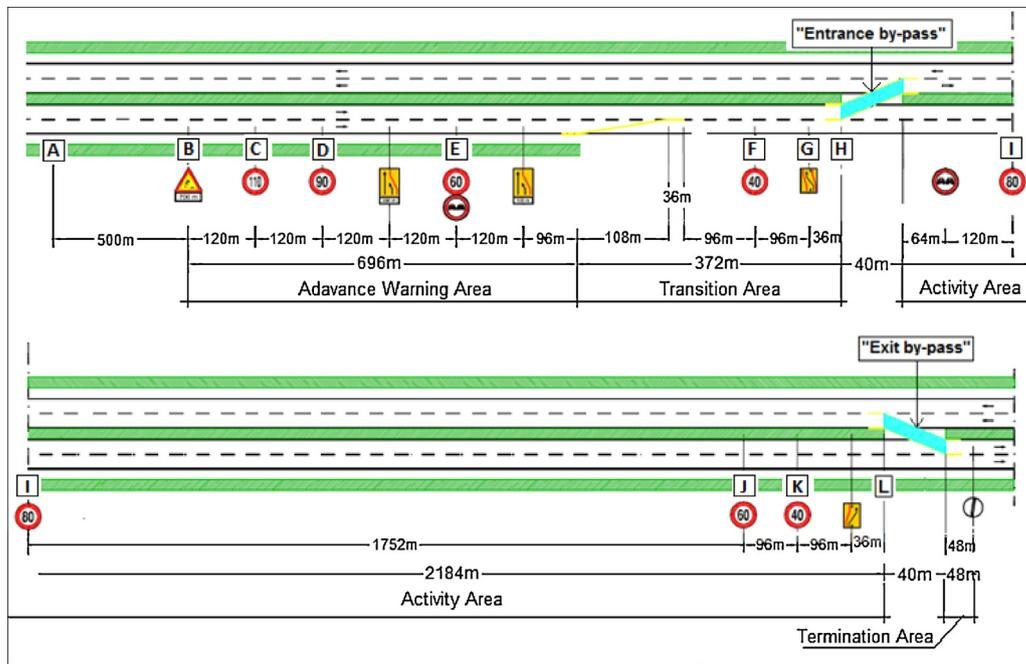
Fig. 5. Speed measurement sites (configuration "0").
