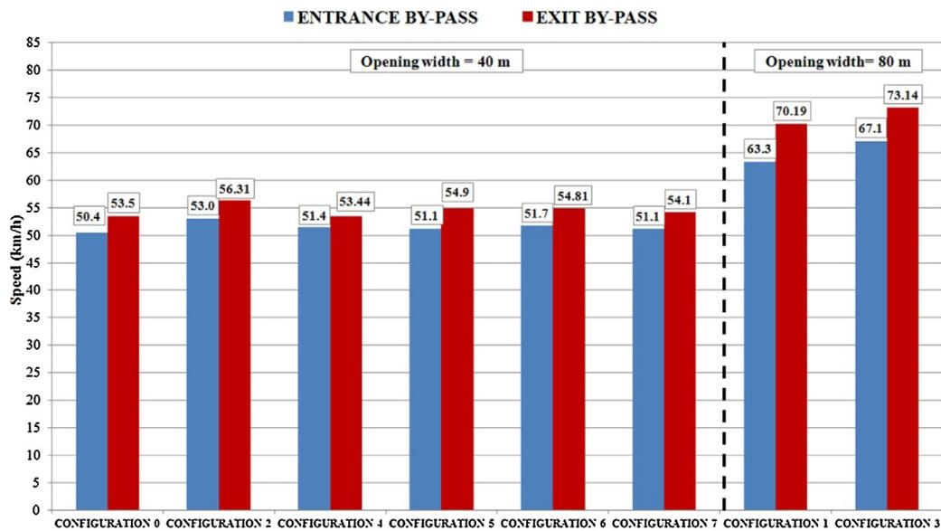
Fig. 14. Mean speeds within the by-passes for the different configurations.
