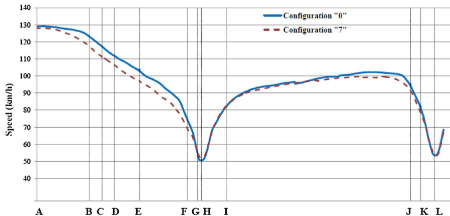
Fig. 11. Comparison between mean speeds profiles (configurations "7" and "0").
