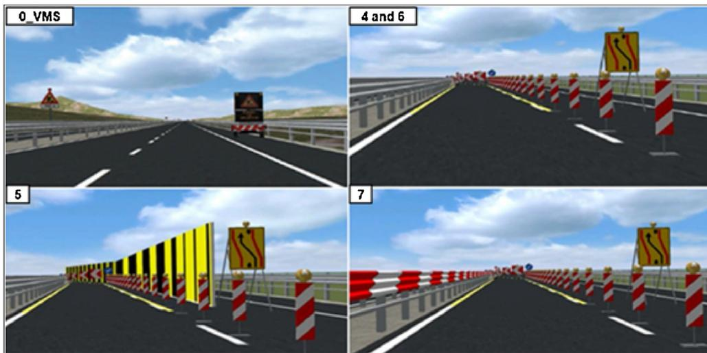
Fig. 4. Images of some work zone’s configurations in the transition area.
