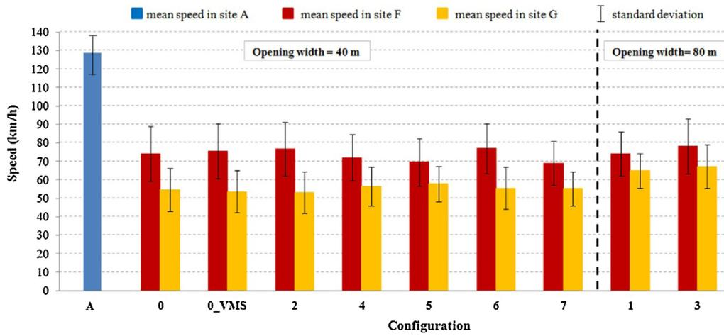
Fig. 13. Mean speeds upstream and in the proximity of the entrance by-pass.
