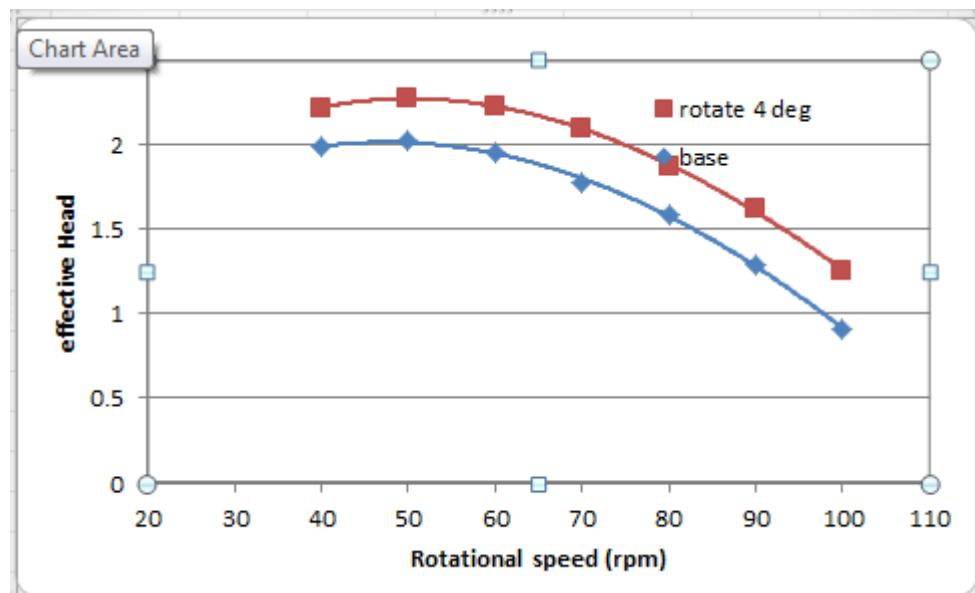
**Figure 4-9 efficient head curve based on rotational speed.**
