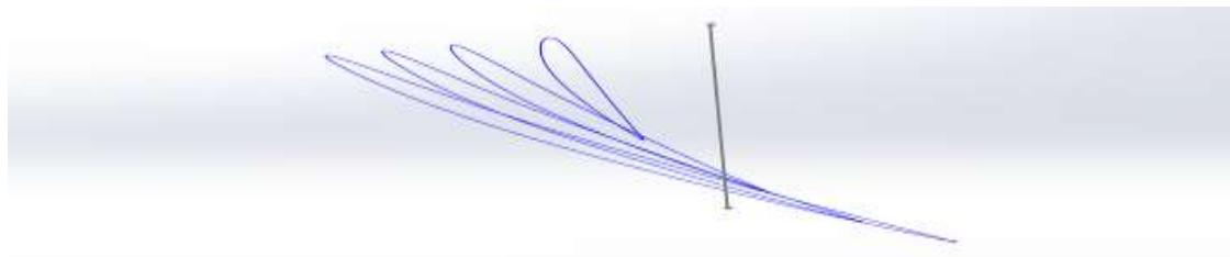
**Figure 3-9 airfoils placed with desired Stagger angle and chord length and their position in relation to rotation axis.**
