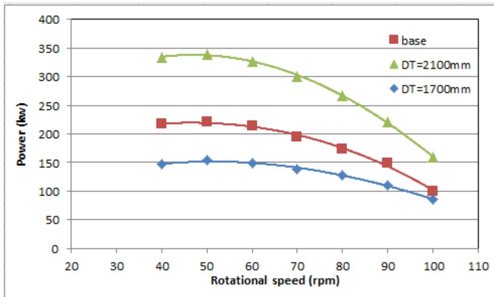
Figure 4-15 power curve based on rotational speed with different tips.
