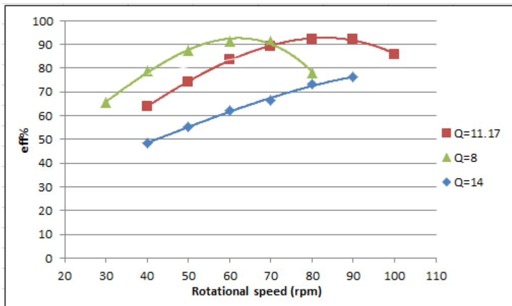
Figure 4-11 efficiency curve based on rotational speed at different flows for the initial turbine
