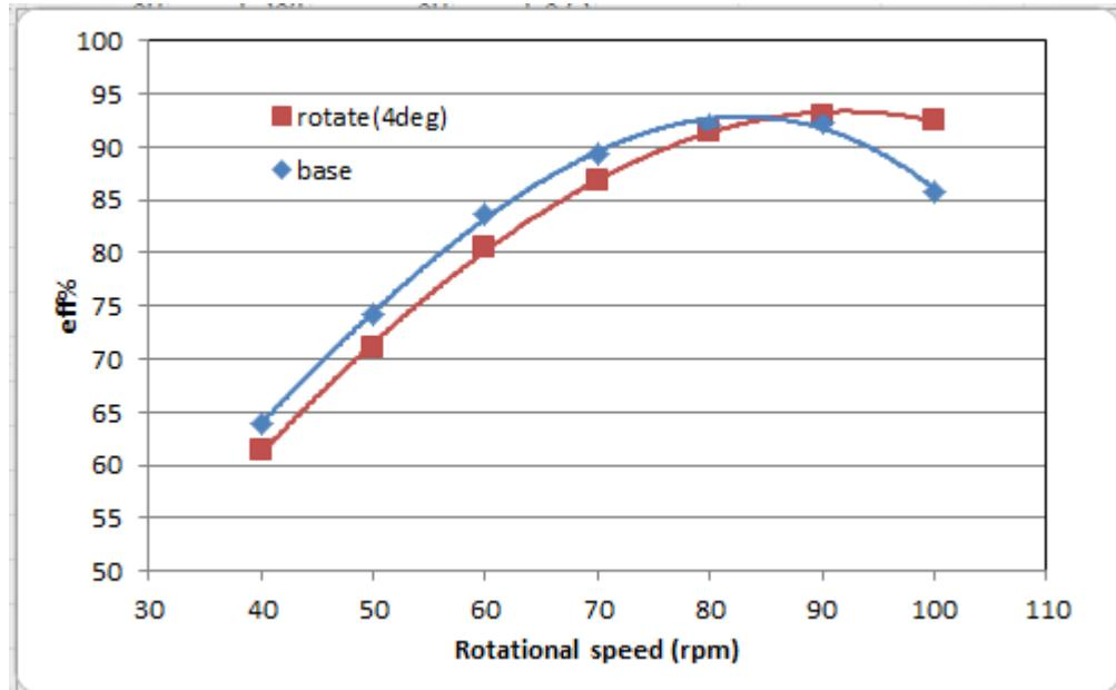
**Figure 4-8 efficiency curve for  $11.17 \text{ m}^3/\text{s}$  flow**
