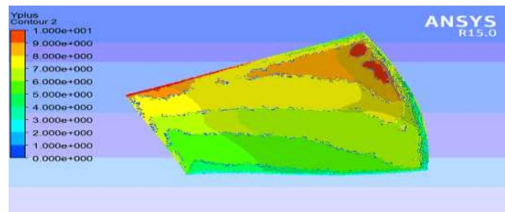
Figure 4-7  $Y^+$  contour on the blade.
