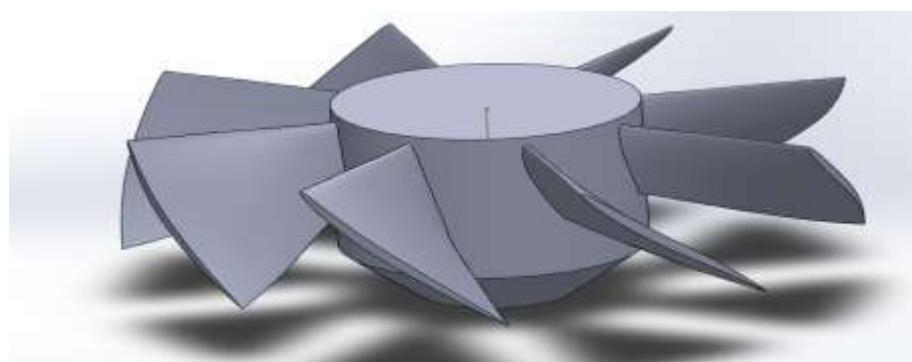
**Figure 3-11 complete turbine rotor with 8 blades.**
