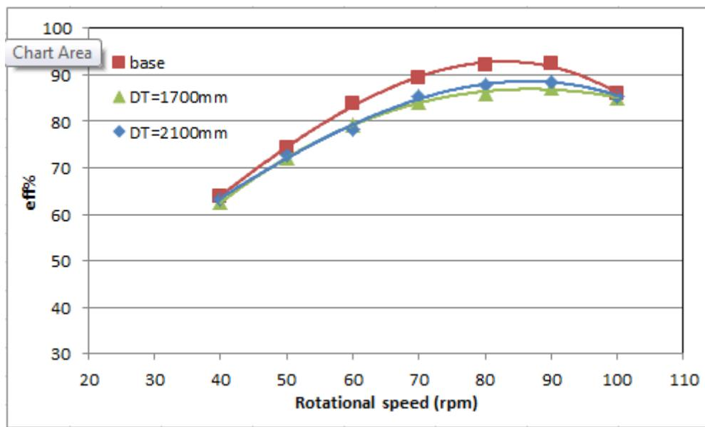
Figure 4-14 efficiency curve based on rotational speed with different tips.
