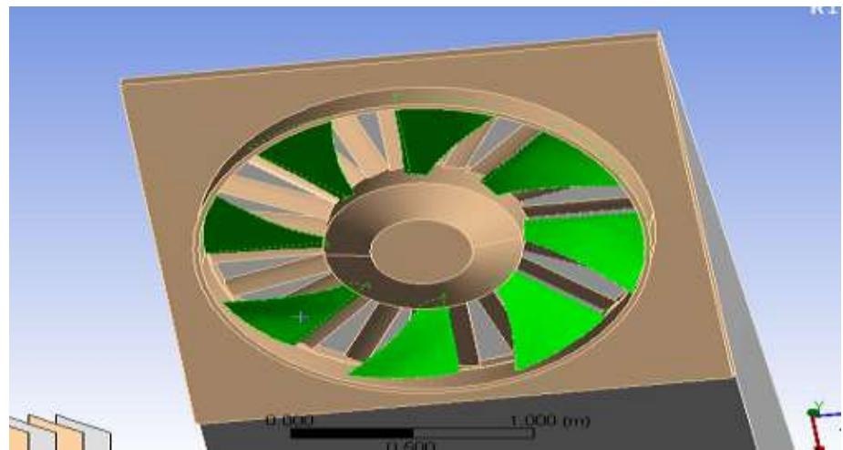
**Figure 3-13 runner blades and their position in relation to fixed turbine chamber.**
