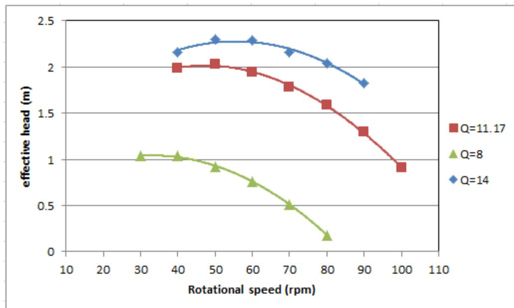
**Figure 4-13** efficient head curve based on rotational speed at different flows for the initial turbine.
