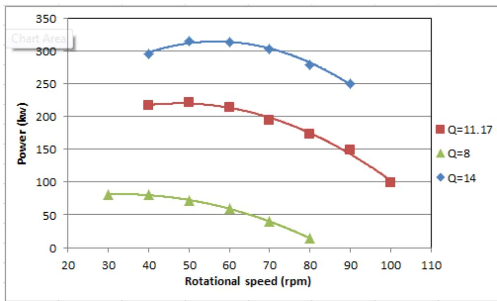
**Figure 4-12** power curve based on rotational speed at different flows for the initial turbine.
