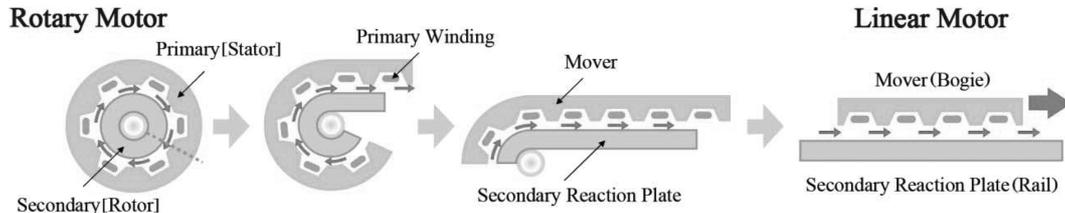
Fig. 1 Concept of a linear motor from a rotary motor [4]
