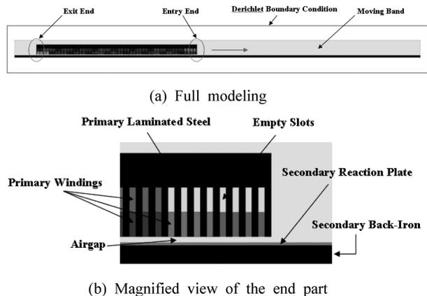
Fig. 6 2-dimensional transient analysis model
