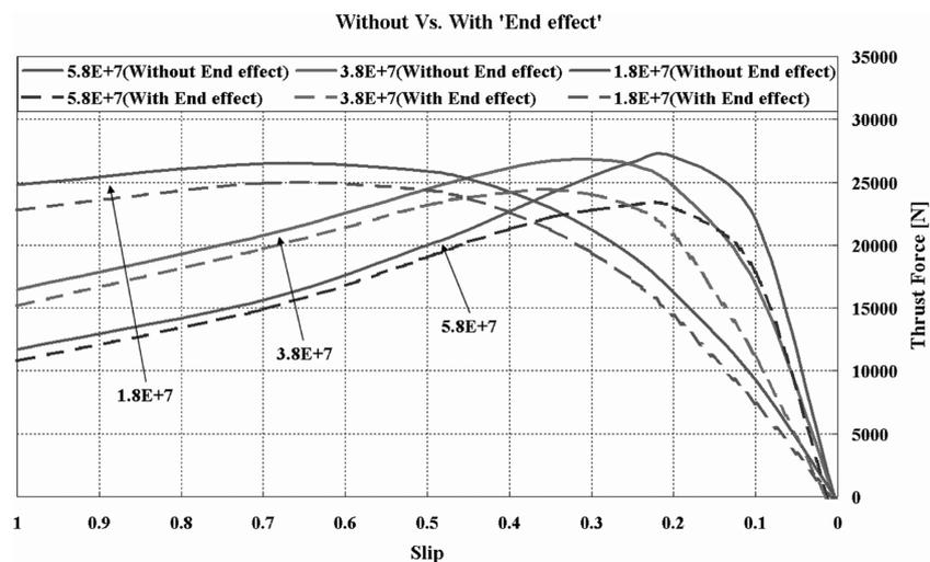
Fig. 8 Thrust force considering without & with 'End effect'
