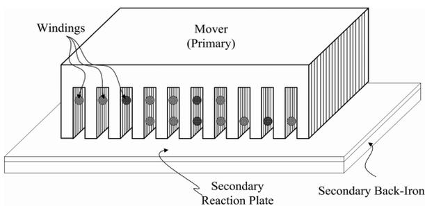
(a) Configuration of a SP type linear induction motor
