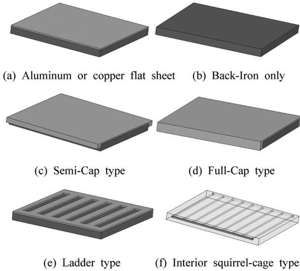
Fig. 3 Various configurations of the secondary reaction plate
