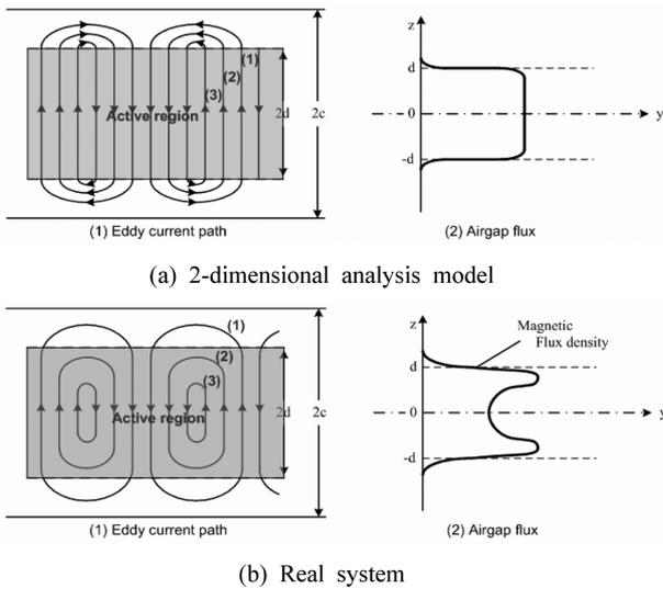
Fig. 4 Magnetic flux density of the 2D analysis and real system
