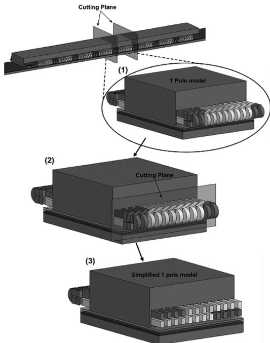
Fig. 7 3-dimensional one pole model (Extracting process from the full model)
