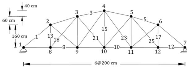
Figure 1: Geometry of bowstring truss.
