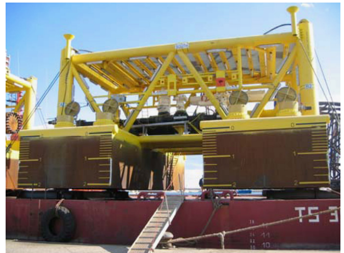
Fig. 8. Skirted shallow foundation for subsea facility (courtesy of Ian Finnie, Advanced Geomechanics).
