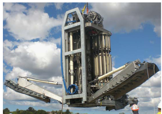
Fig. 2. Photograph of the second generation PROD (courtesy Benthic Geotech).
