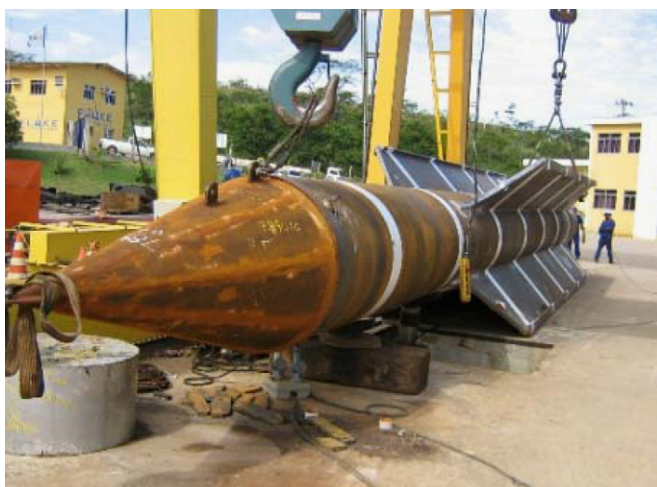
Fig. 14. Typical torpedo anchors with four flukes (after de Aguiar et al., 2009).
