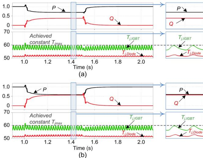
Fig. 15. Performance of a 1-kW single-phase PV inverter with  $T$ -optimized strategy under grid faults (active power  $P$  and reactive power  $Q$  [p.u.]; junction temperature  $T_j$  [°C];  $v_g = 0.75$  p.u.): (a)  $k = 2$  p.u. and (b)  $k = 3$  p.u.
