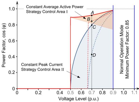
Fig. 9. Power factor curves versus voltage levels for different control strategies. Solid lines:  $k = 2$ . Dashed lines:  $k = 3$ .  $k$  is defined in (1).
