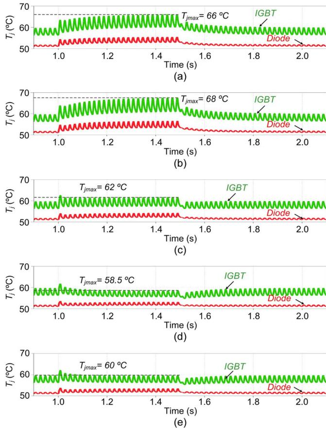
Fig. 16. Junction temperature ( $T_j$ ) of the power devices in a 1-kW single-phase PV inverter under grid faults (voltage level  $v_g = 0.55$  p.u. and  $k = 2$  p.u.): (a) Without LVRT, (b) *Const.-P* with  $k_d = 1$  p.u., (c) *Const.-I<sub>d</sub>* with  $m = 1$  p.u., (d) *Const.-I<sub>g max</sub>* with  $n = 1$  p.u., and (e) *T-optimized*.
