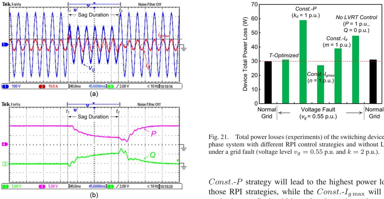
Fig. 20. Experimental results of a 1-kW single-phase system with *T-Optimized* RPI control strategy (voltage level  $v_g = 0.55$  p.u. and  $k = 2$  p.u.): (a) Grid voltage  $v_g$  [100 V/div] and grid current  $i_g$  [10 A/div]; (b) active power  $P$  [500 W/div] and reactive power  $Q$  [500 var/div]; time [40 ms/div].
