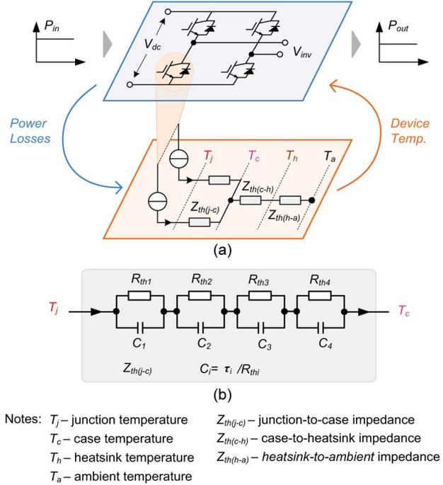
Fig. 8. (a) Electrical and thermal models of a power module and (b) Foster model of the thermal impedance from junction to case [47], [51], [52].
