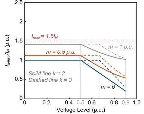
Fig. 6. Design constraint of the *Const.-I<sub>d</sub>* considering the inverter overcurrent protection, where  $m = I_d/I_N$  and  $k$  is defined in (1).
