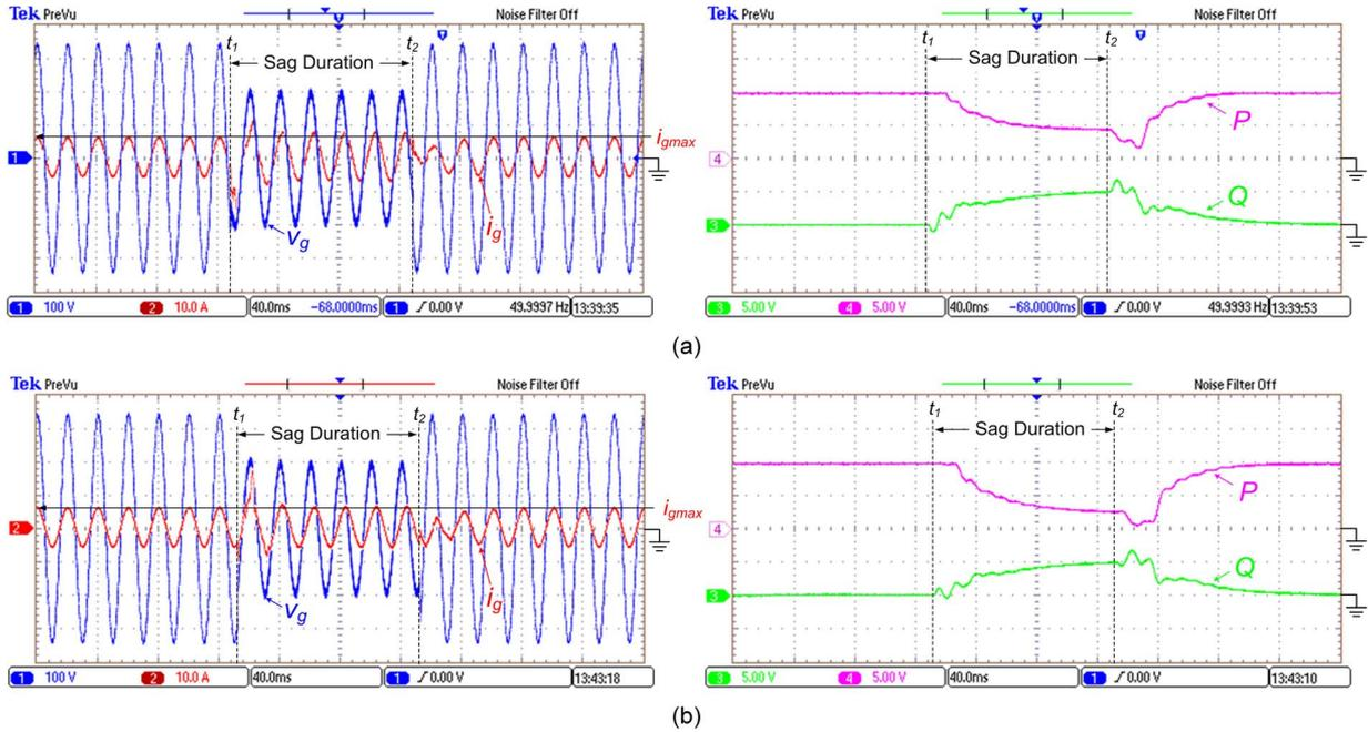
Fig. 19. Experimental results of a single-phase grid-connected system with different RPI control strategies (voltage level  $v_g = 0.55$  p.u.,  $k = 2$  p.u., grid voltage  $v_g$  [100 V/div], grid current  $i_g$  [10 A/div], active power  $P$  [500 W/div], reactive power  $Q$  [500 var/div], and time [40 ms/div]): (a) *Const.-I<sub>d</sub>* with  $m = 1$  p.u. and (b) *Const.-I<sub>gmax</sub>* with  $n = 1$  p.u.
