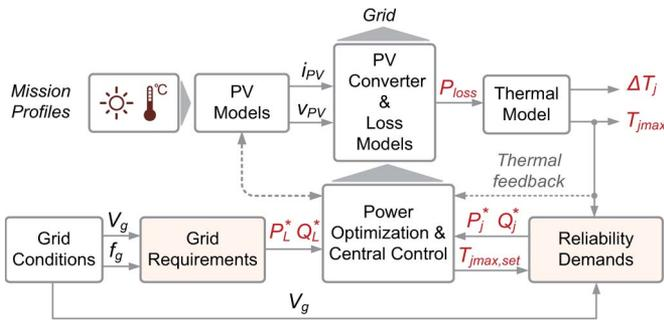
Fig. 10. Control structure of the  $T$ -Optimized strategy for single-phase PV systems.
