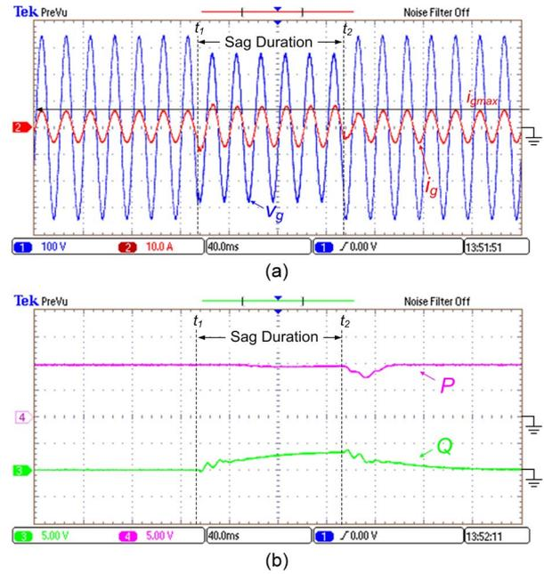
Fig. 18. Experimental results of a single-phase system with the *Const.-P* RPI control strategy (voltage level  $v_g = 0.8$  p.u.,  $k_d = 1$  p.u., and  $k = 2$  p.u.): (a) Grid voltage  $v_g$  [100 V/div] and grid current  $i_g$  [10 A/div]; (b) active power  $P$  [500 W/div] and reactive power  $Q$  [500 var/div]; time [40 ms/div].
