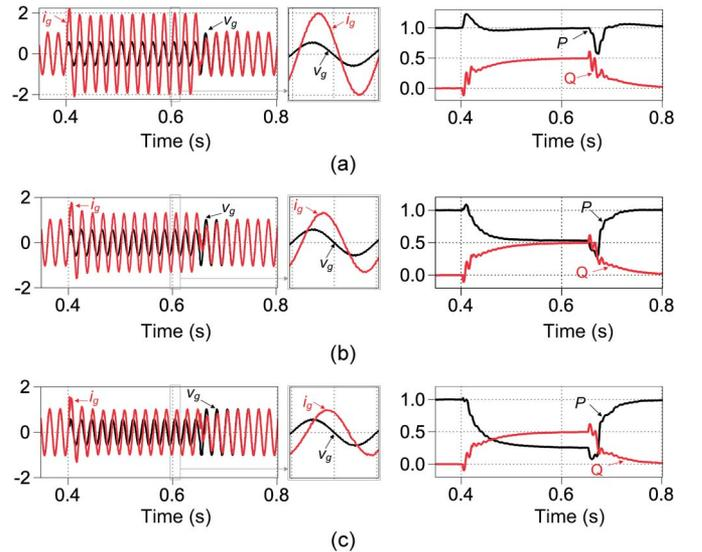
Fig. 13. Performance of a 1-kW single-phase PV system in LVRT operation mode with three different RPI control strategies ( $i_g$ ,  $v_g$ —grid current and voltage [p.u.];  $P$ ,  $Q$ —average active power and reactive power [p.u.]; voltage level:  $v_g = 0.55$  p.u.;  $k = 2$  p.u.): (a) *Const.-P* with  $k_d = 1$  p.u., (b) *Const.-I<sub>d</sub>* with  $m = 1$  p.u., and (c) *Const.-I<sub>gmax</sub>* with  $n = 1$  p.u.
