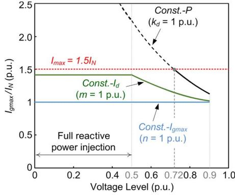
Fig. 7. Application conditions for three RPI strategies under different grid voltage levels for the case when  $k = 2$  p.u. and  $I_{\max} = 1.5I_N$ .
