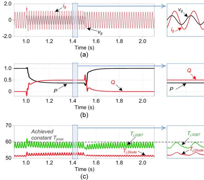
Fig. 14. Simulation results of a 1-kW single-phase grid-connected PV system with  $T$ -optimized control strategy ( $k = 2$  p.u.): (a) Grid current  $i_g$  and voltage  $v_g$  [p.u.], (b) active power  $P$  and reactive power  $Q$  [p.u.], and (c) junction temperature  $T_j$  [°C]; voltage level:  $v_g = 0.55$  p.u.
