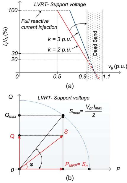
Fig. 4. Reactive power profiles for single-phase systems: (a) During LVRT for medium- and/or high-voltage systems [29], [31], [43] and (b) reactive power capability of a PV inverter.
