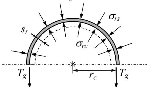
Figure 2. Equilibrium and compatibility conditions of the encasement.
