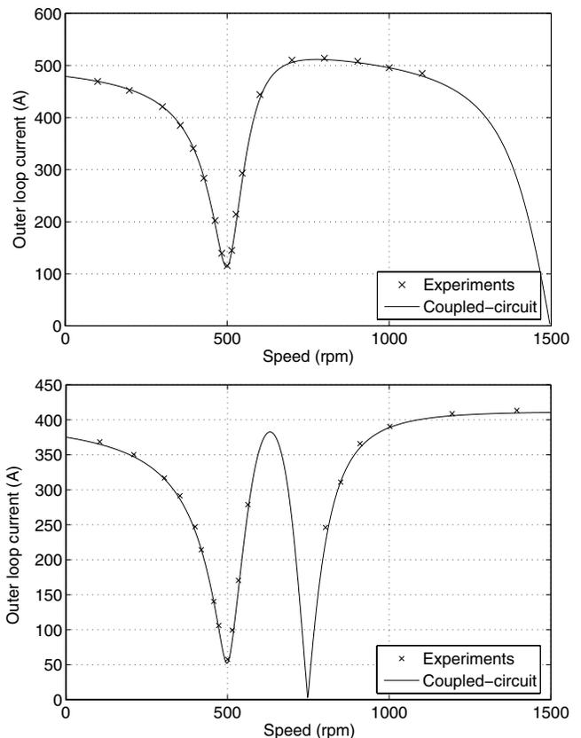
Fig. 10. Rotor outer-loop current in the cascade mode of operation.
