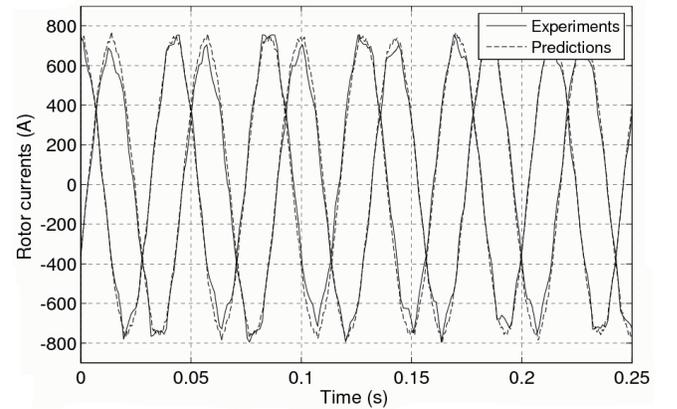
Fig. 8. Outer loop currents for two consecutive nests of the nested-loop rotor.
