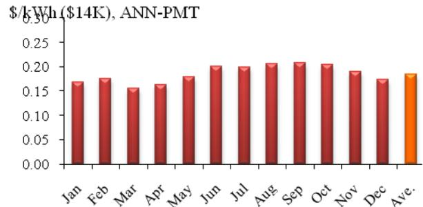
Fig. 5 PV Electricity cost, \$14K, mortgage: 6%
