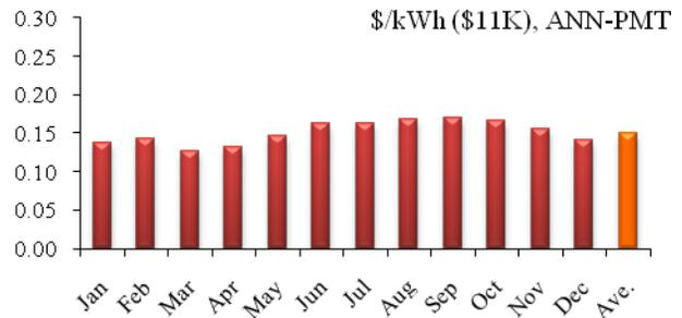
Fig. 6 PV Electricity cost, \$11K, mortgage: 6%
