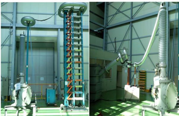
Fig. 9. LI and AC Test layout
