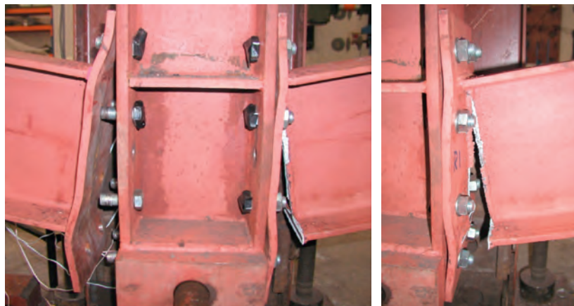
(a) Failed connection (b) Fracture of weld
