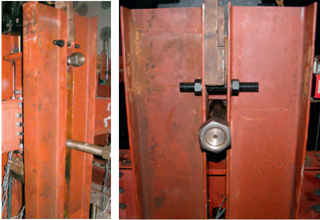
(a) Rotational restraint system
