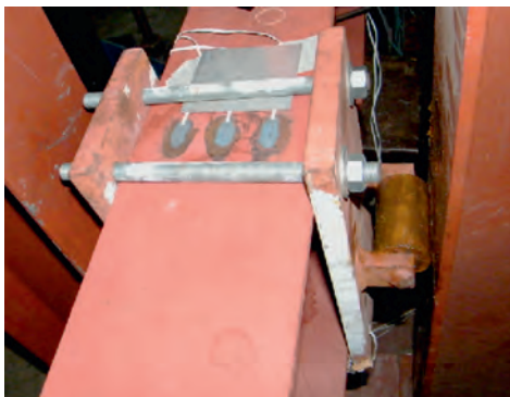
(b) Lateral restraint system
