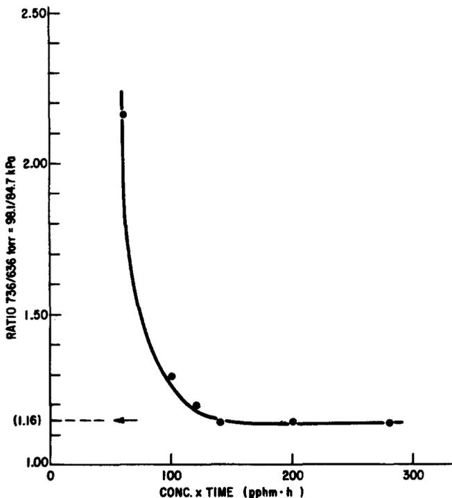
Fig. 6. Log (SOC) ratio at 736 torr (98.1 kPa)/636 torr (84.7 kPa) v. the severity of ozone exposure, i.e.  $O_3$  concentration  $\times$  time.
