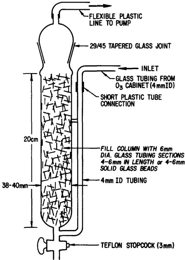
Fig. A.1. Ozone absorption column as used in inter-laboratory program.
