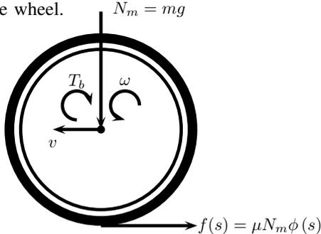
Fig. 2. Wheel forces and torques
