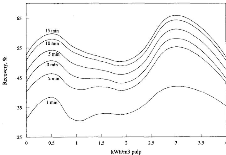
Fig. 3. Gold flotation recovery as a function of time and shear energy transferred in the conditioning stage. Pine oil, 72 g/t as frother and 120 g/t amyl xanthate as collector.
