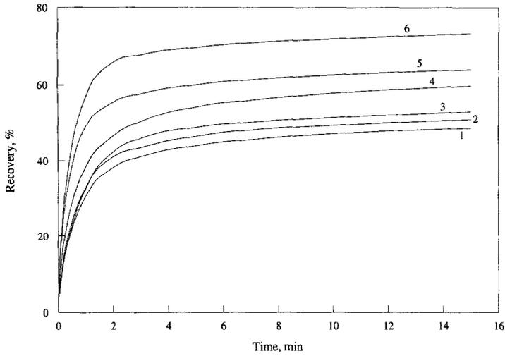
Fig. 9. Effect of frother type on flotation kinetics of gold particles as a function of shear energy in the conditioning stage. 120 g/t amyl xanthate as collector and 72 g/t the frother concentration. 1 = MIBC: 2 kWh/m<sup>3</sup> pulp; 2 = pine oil: 2 kWh/m<sup>3</sup> pulp; 3 = MIBC: 0.5 kWh/m<sup>3</sup> pulp; 4 = pine oil: 0.5 kWh/m<sup>3</sup> pulp; 5 = Dowfroth 1012: 0.5 kWh/m<sup>3</sup> pulp and 6 = Dowfroth 1012: 2 kWh/m<sup>3</sup> pulp.
