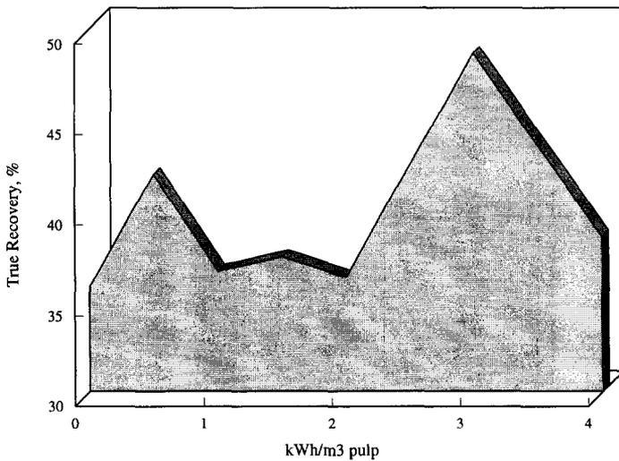
Fig. 6. Effect of HIC on gold true flotation recovery. Pine oil, 72 g/t as frother and 120 g/t amyl xanthate as collector.
