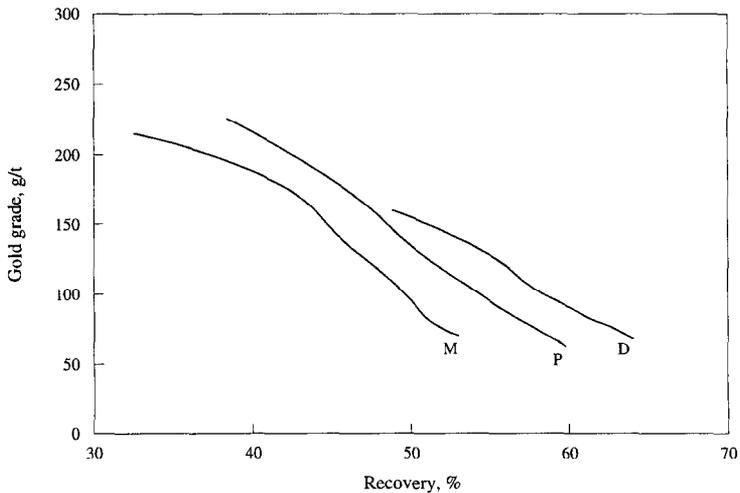
Fig. 10. Grade–recovery flotation curves for different frothers. HIC = 0.5 kWh/m<sup>3</sup> pulp; 120 g/t amyl xanthate as collector and 72 g/t the frother concentration. D = Dowfroth 1012; P = pine oil and M = MIBC.
