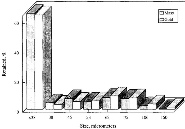
Fig. 1. Gold and particle size distribution in feed.
