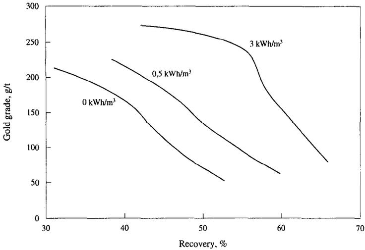
Fig. 5. Grade–recovery flotation curves with and without HIC. Pine oil, 72 g/t as frother and 120 g/t amyl xanthate as collector.
