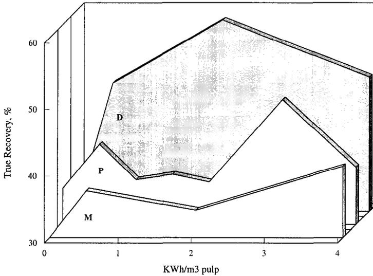
Fig. 11. Effect of HIC on true gold recovery values for different frothers. 120 g/t amyl xanthate as collector and 72 g/t the frother concentration. *D* = Dowfroth 1012; *P* = pine oil and *M* = MIBC.
