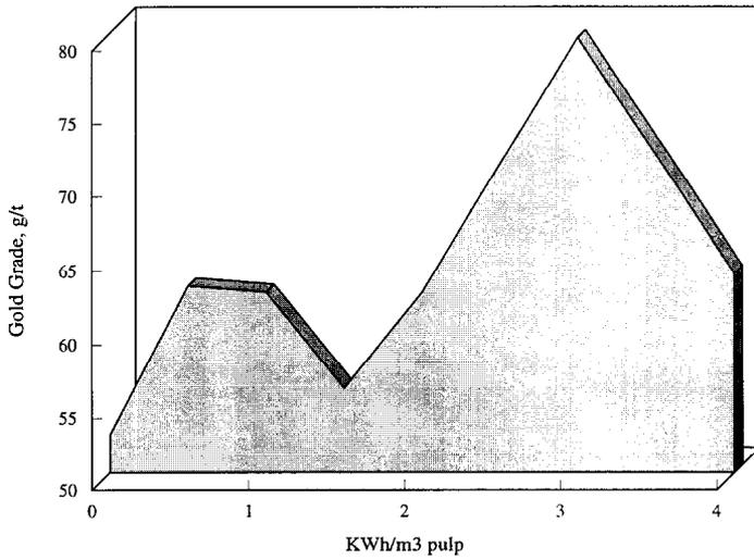
Fig. 7. Effect of HIC on concentrate gold grade. Pine oil, 72 g/t as frother and 120 g/t amyl xanthate as collector.
