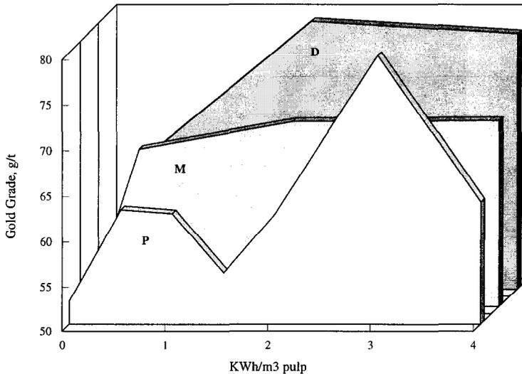
Fig. 12. Effect of HIC on concentrate gold grade for different frothers. 120 g/t amyl xanthate as collector and 72 g/t the frother concentration. *D* = Dowfroth 1012; *P* = pine oil and *M* = MIBC.
