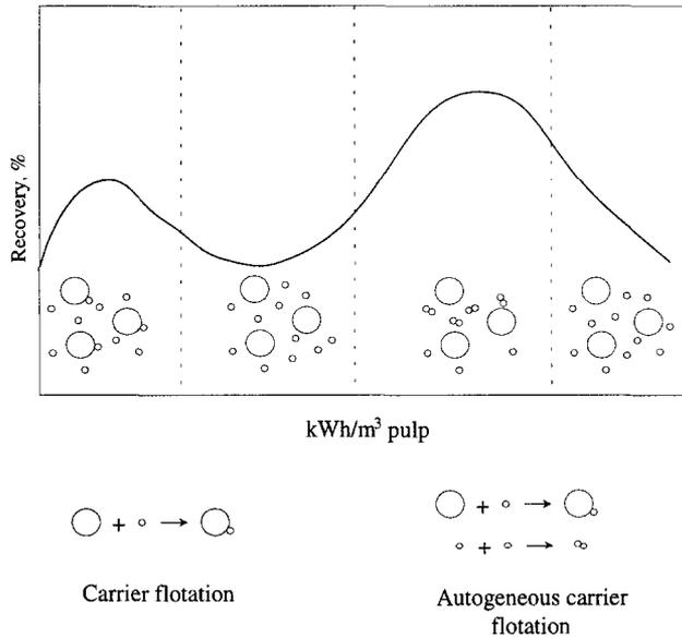
Fig. 4. Particle aggregation phenomena during the conditioning stage and mechanisms of flotation.
