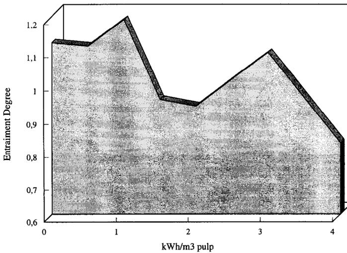
Fig. 8. Effect of HIC on the degree of gold values entrainment. Pine oil, 72 g/t as frother and 120 g/t amyl xanthate as collector.
