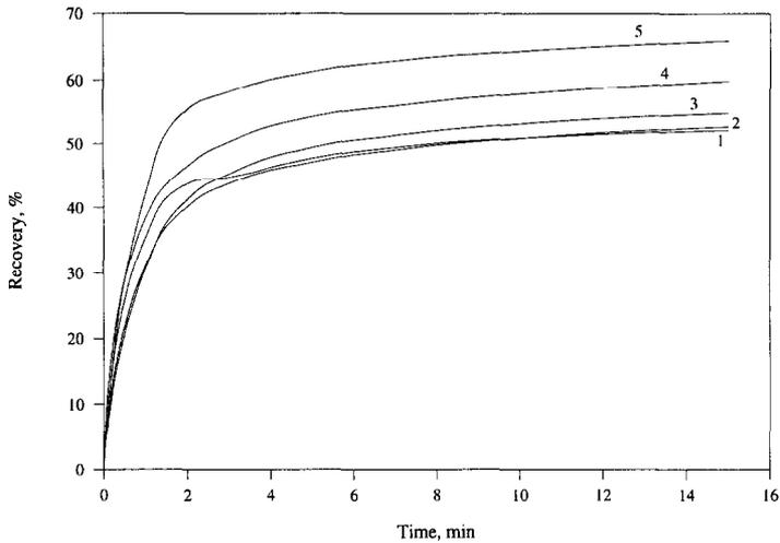
Fig. 2. Flotation kinetics of gold particles as a function of the energy transferred during HIC. Pine oil, 72 g/t as frother and 120 g/t amyl xanthate as collector. 1 = 0; 2 = 4; 3 = 1; 4 = 0.5 and 5 = 3 kWh/m<sup>3</sup> pulp.
