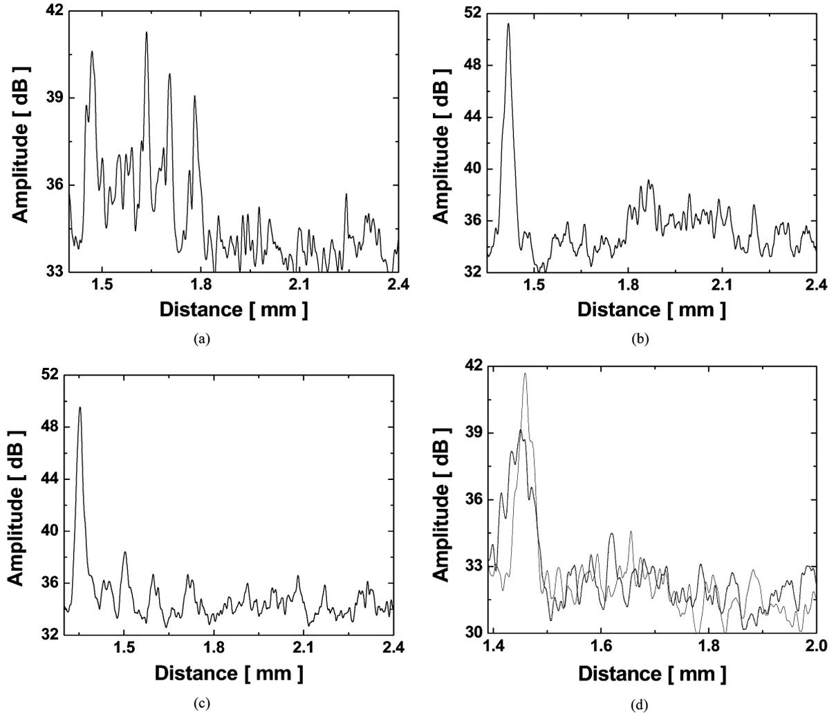
Fig. 5. Captured image using a gold-coated side-viewing fiber tip: (a) polymer tape layers; (b) IR sensing card (single polymer layer + organic material); (c) onion skin; (d) Rat brain (solid line: normal, dotted line: tumor).
