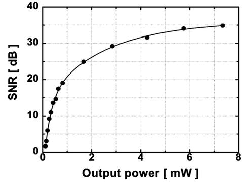
Fig. 3. SNR versus output power: circle-measured, solid line-fitted trend curve.
