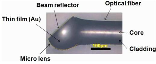
Fig. 1. Example photo of the fabricated thin-film gold-coated side-viewing fiber-optic imaging microprobe and its layout.
