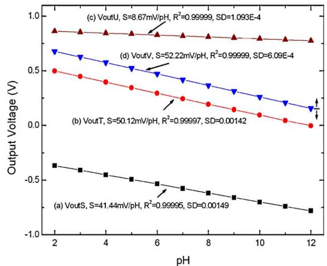
Fig. 5. Simulation plots of the output signal of the proposed body-effect reduction circuit for pH sweep.
