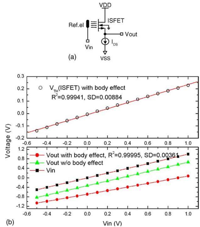
Fig. 1. (a) A n-channel depletion ISFET; (b) input and output voltages with and without (w/o) body effect.
