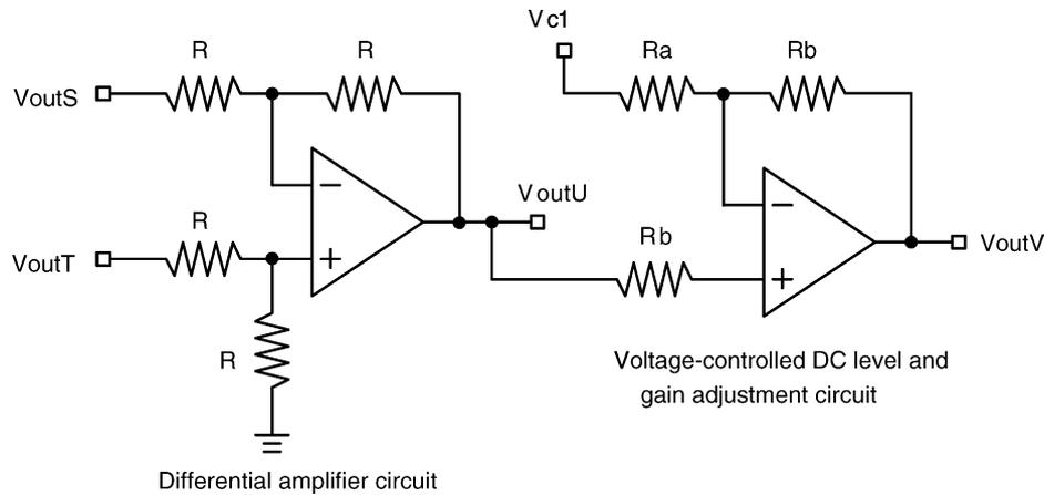
Fig. 4. Circuit for ISFET performance enhancement.
