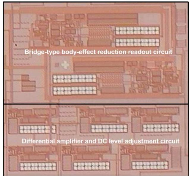
Fig. 8. Chip microphotography of the total body-effect reduction and performance enhancement circuitry.
