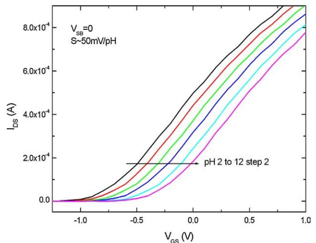
Fig. 9.  $I_{DS}$  vs.  $V_{GS}$  characteristics of an ISFET operating in the proposed circuit for buffer solutions of different pH and for  $V_{SB} = 0$ .
