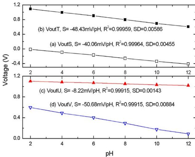
Fig. 10. pH response of ISFET operating in the body-effect reduction circuit with the ISFET bulk connected to VSS.
