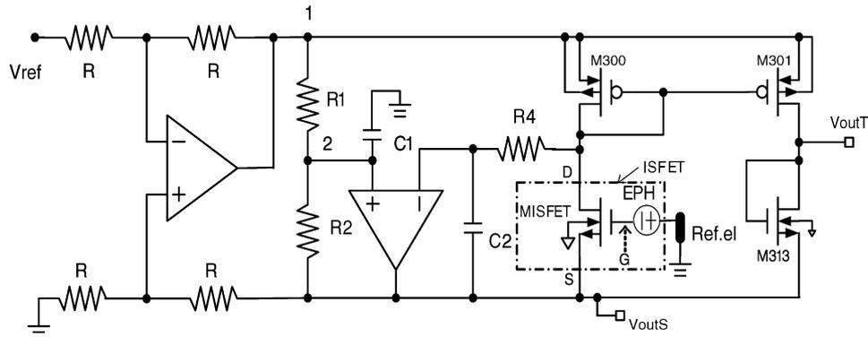
Fig. 3. Diagram of the bridge-type body-effect reduction readout interface.
