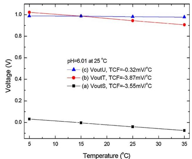
Fig. 12. Output voltage vs. temperature for ISFETs operated by a circuit with/without compensation.
