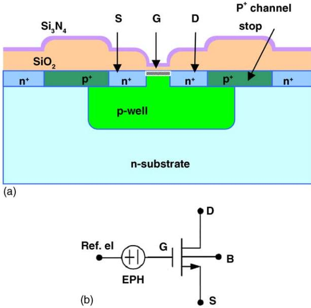
Fig. 2. (a) ISFET structure layout; (b) equivalent sub-circuit block of the ISFET macro-model.
