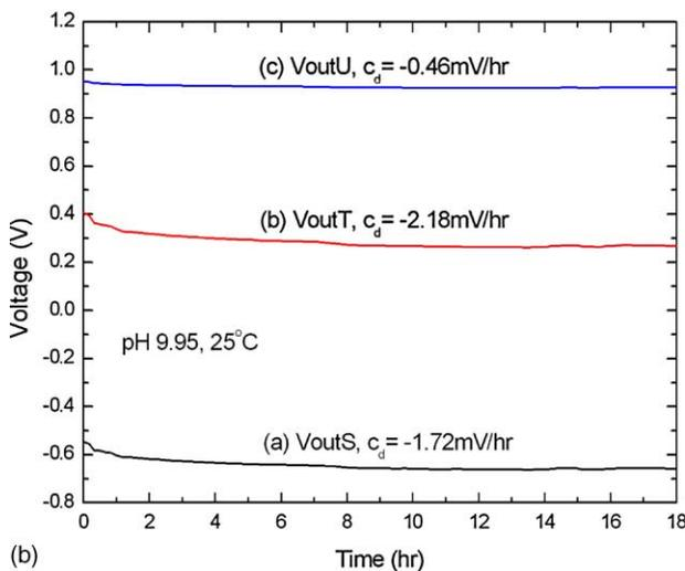
Fig. 11. Time-dependency response with and without differential compensation methods.
