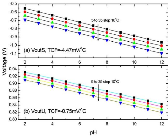
Fig. 6. Simulation of ISFET interfacial voltage in the pH range of 2–12 for the temperature range of 5–35 °C.
