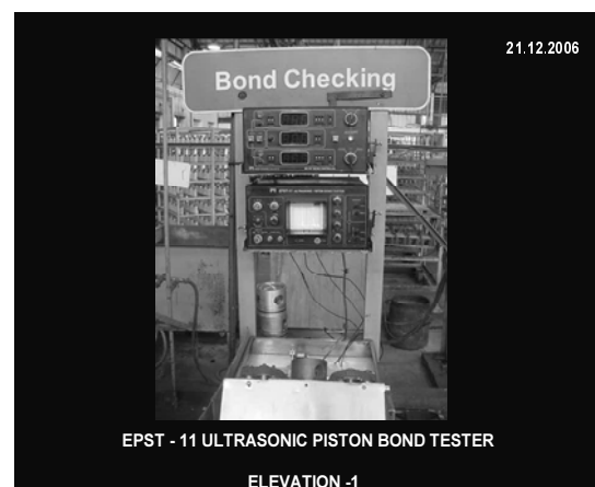
Fig. 8 Ultrasonic bond-checking facility
