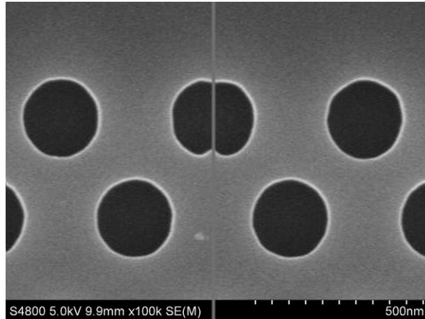
Fig. 2. SEM micrograph of the PhC structure at the writefield edge. The grey line represents the writefield boundary and a small deformation of the hole is apparent.
