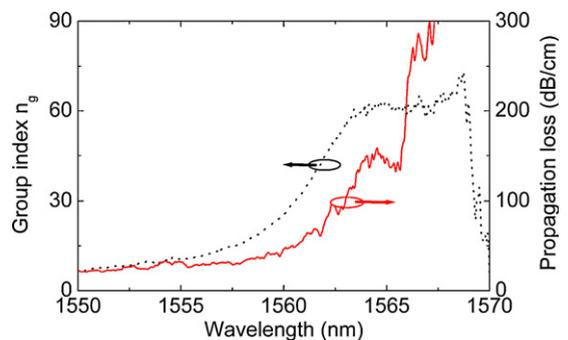
Fig. 3. Measured propagation loss (red solid line), and group index (black dotted line) of the slow light PhC waveguides with SFS mode conversion interface. (For interpretation of the references to colour in this figure legend, the reader is referred to the web version of the article.)
