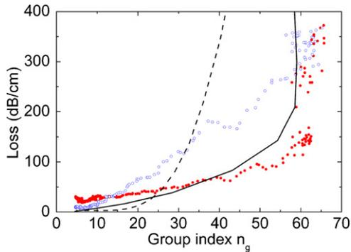
Fig. 4. Experimentally measured propagation loss of the slow light waveguide as a function of group index with (red solid dots) and without (blue open circles) SFS mode conversion interface. The solid line is the simulation result without any stitching errors. The dashed line shows the simulated results for a W1 waveguide. (For interpretation of the references to colour in this figure legend, the reader is referred to the web version of the article.)
