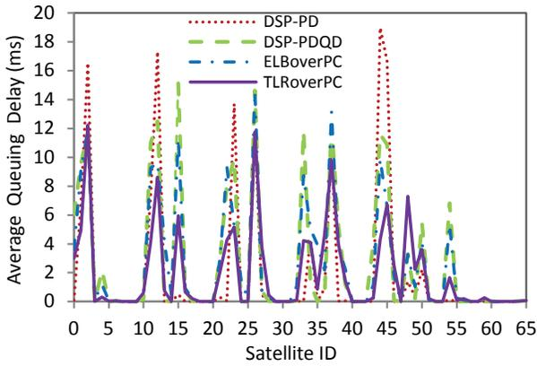
Fig. 11: Average queuing delay at each satellite.
