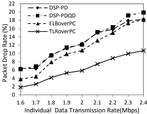
Fig. 12: Packet drops for different sending rates.
