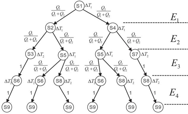
Fig. 7: Transmitting route from  $S_1$  to  $S_9$ .
