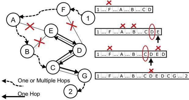
Fig. 5: Endless-loop-free mechanism.
