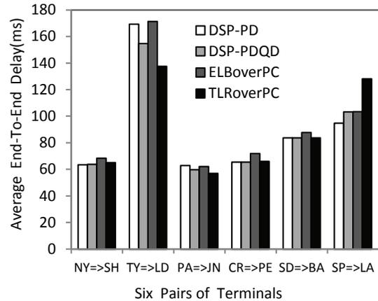
Fig. 10: Average end-to-end delay of six terminal pairs.
