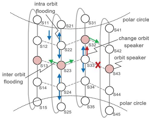
Fig. 4: Advanced orbit speaker mechanism.
