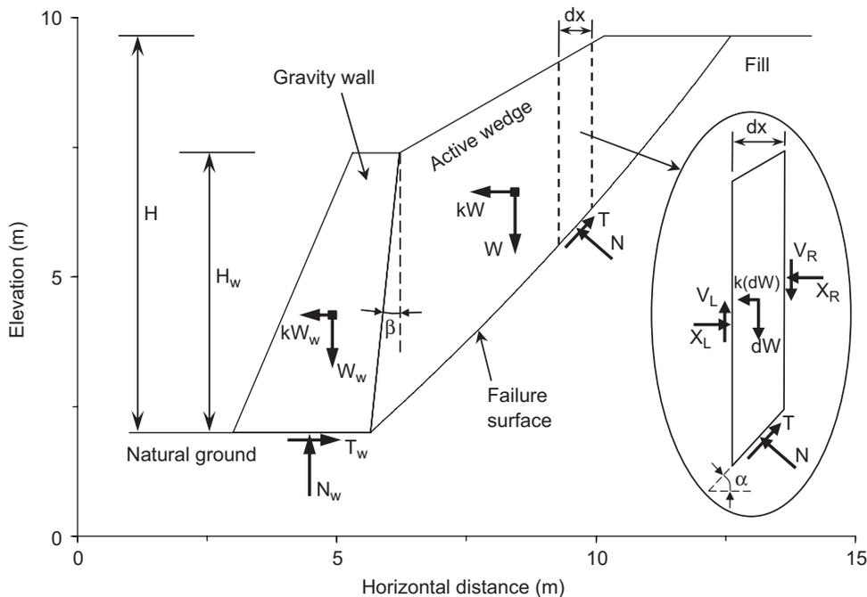
Fig. 3. Forces considered in the seismic sliding block analysis of the gravity retaining wall–active wedge system.
