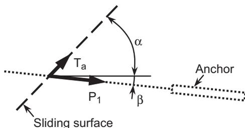
Fig. 9. Equivalent system of forces considered in the pseudostatic *SLOPE/W* stability analysis of the anchor-reinforced slope to account for the modified reinforcement approach.
