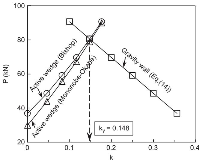
Fig. 6. Graphical procedure to determine the yield coefficient ( $k_y$ ) of the gravity wall–backfill system based on the  $P$ – $k$  relationships at limit equilibrium established independently for the gravity retaining wall and the soil active wedge behind the wall.
