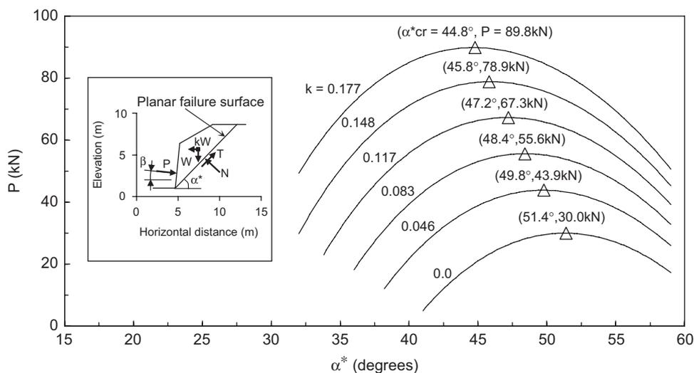
Fig. 7. Mononobe–Okabe analysis to evaluate the dynamic wall thrust ( $P$ ) and inclination of critical failure plane ( $\alpha_{cr}^*$ ) for different seismic coefficients ( $k$ ).
