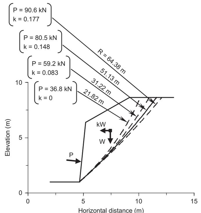
Fig. 5. Critical circular slip surfaces for various magnitudes of dynamic wall thrust ( $P$ ) and corresponding seismic coefficients ( $k$ ) at limit equilibrium of the active wedge (i.e.,  $FS = 1.0$ ).
