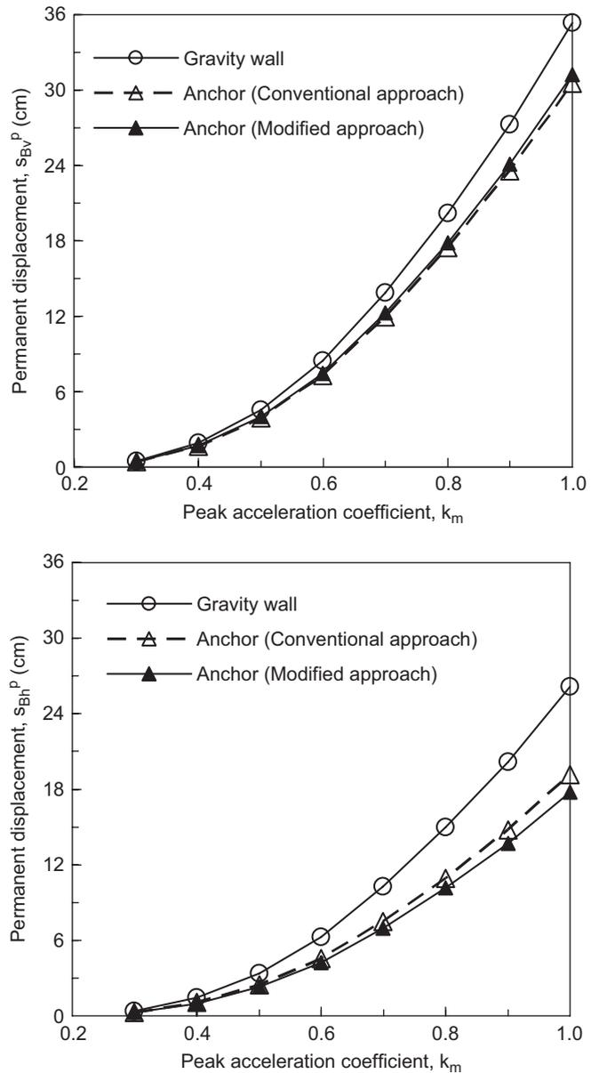
Fig. 12. Permanent vertical ( $s_{Bv}^p$ ) and horizontal ( $s_{Bh}^p$ ) seismic displacements at the top of the sliding soil mass within the fill slope supported by gravity retaining wall or reinforced with anchors, in relation to the peak earthquake acceleration coefficient ( $k_m$ ).
