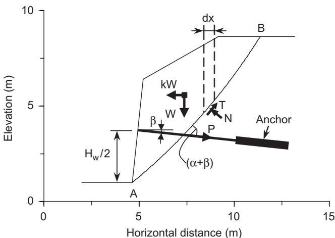
Fig. 8. Forces considered in the seismic sliding block analysis of the anchor-reinforced slope.
