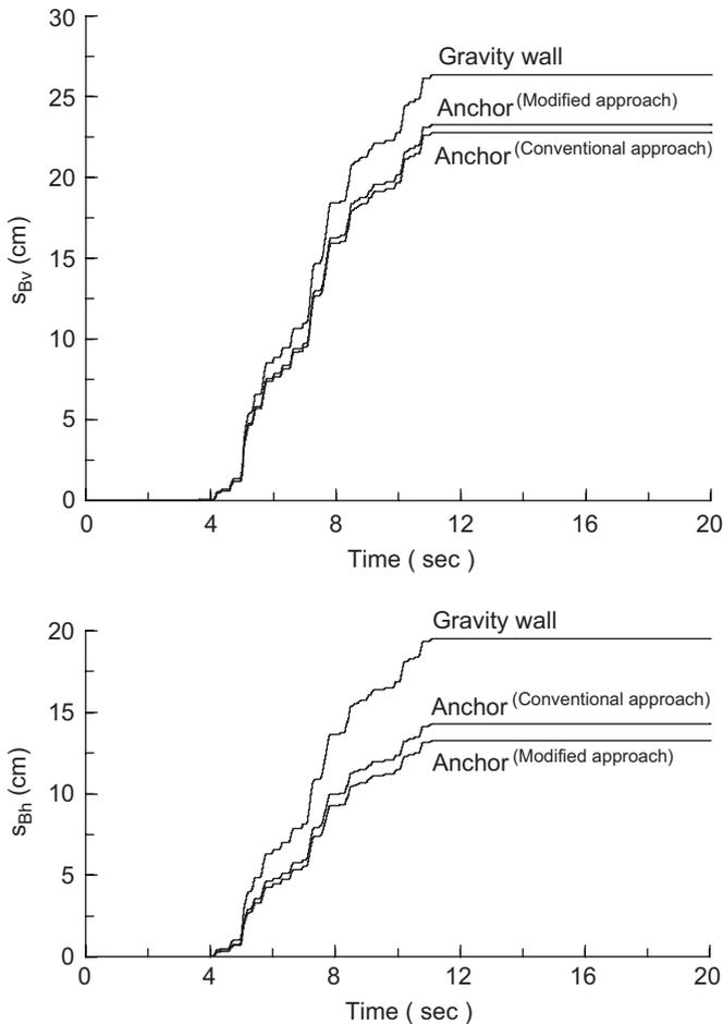
Fig. 11. Evolution of vertical ( $s_{Bv}$ ) and horizontal ( $s_{Bh}$ ) displacements during earthquake at the top of the sliding soil mass within the fill slope supported by gravity retaining wall or reinforced with anchors.
