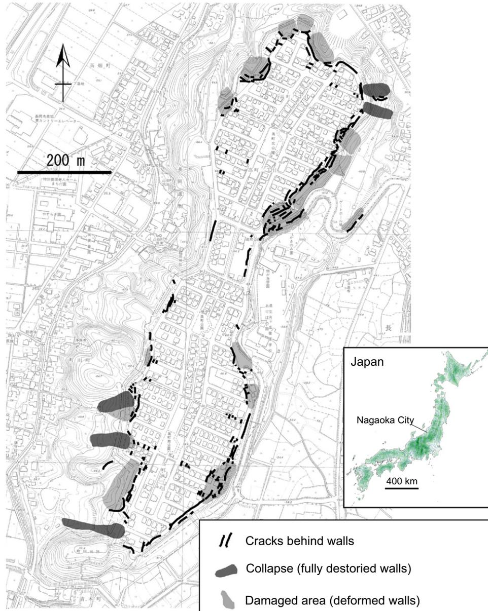
**Fig. 1.** Map of Takamachi-danchi residential area showing the ground failure and gravity retaining wall damage during the October 23, 2004 Chuetsu earthquake, Niigata, Japan.
