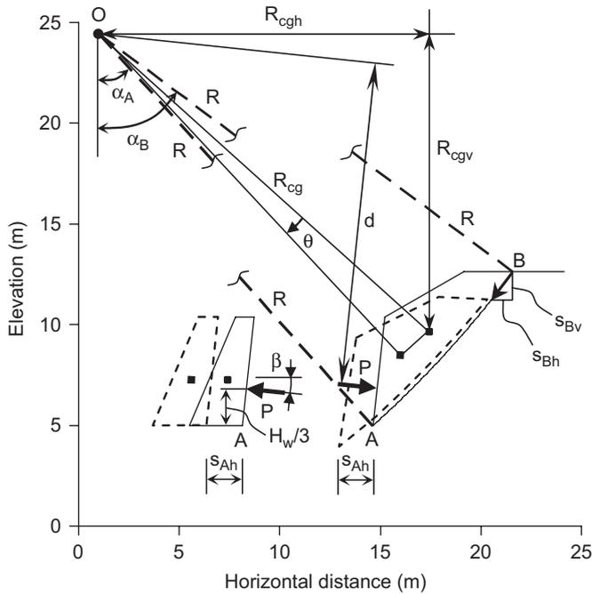
Fig. 4. Illustration of the translational failure mechanism for the gravity retaining wall, and the rotational failure mechanism for the potential sliding soil mass within the fill slope.
