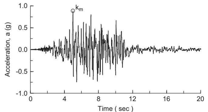
Fig. 10. Input horizontal ground motion.
