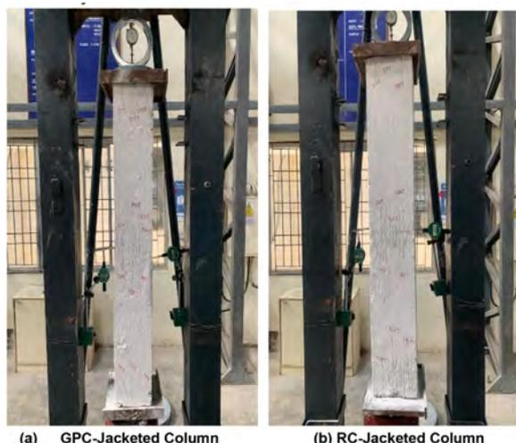
Fig. 19. Failure of GPC & RC-jacketed columns.
