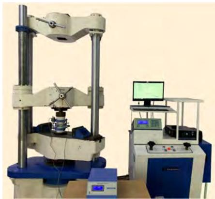
**Fig. 1.** Compression test on concrete cylinder.
