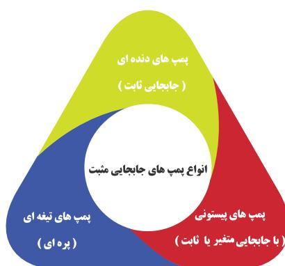
Positive displacement or hydrostatic pumps produce flow proportional to their displacement and rotor speed. The pump output flow is constant and not dependent on system pressure.
