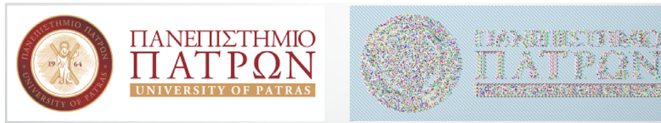
Fig. 9. (a) original image, (b) encrypted image using AES-ECB mode.
