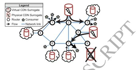
Figure 1: *System model.* The network is composed by consumers, routers, virtual and physical CDN surrogates. Our proposed optimization model selects (1) the planning of physical CDNs and (2) request routing.
