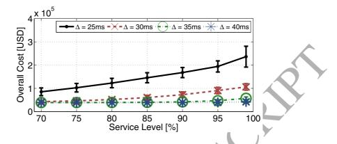
Figure 2: Effect of the Service Level and Delay. The figure shows the overall cost as a function of the desired service level ( $\epsilon$ ) and for different delays ( $\Delta = \{25, 30, 35, 40\}$  ms).
