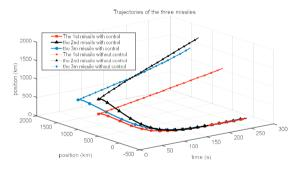
Fig.4. 3D simulation of missiles flight trajectory under large disturbances (with or without control)
