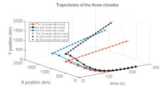
Fig.2. 3D simulation of missiles flight trajectory under small disturbances(with or without control)
