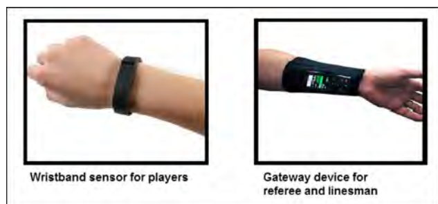
Fig. 13. Wireless device used by the player and Referee/Linesman.
