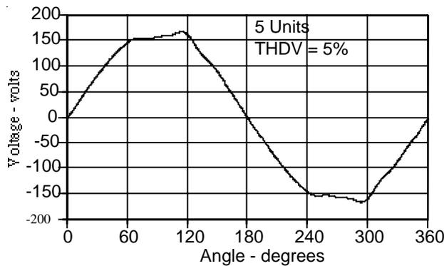
Figure 5: Distortion of Voltage Waveform with N Parallel 100 W Computer Loads
