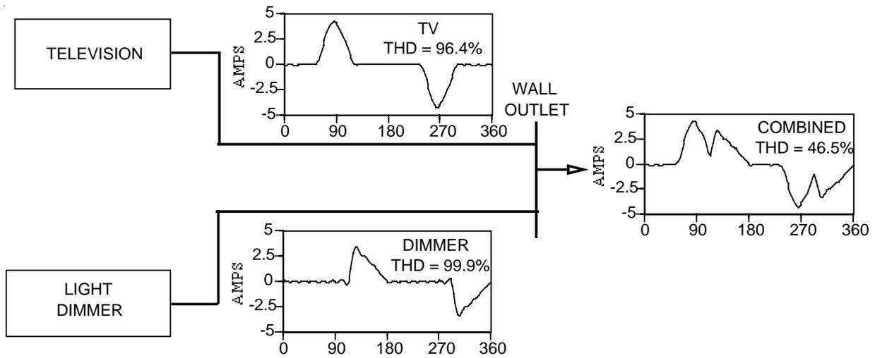
Figure 1. Example of Harmonic Current Phase Angle Cancellation for Television and Light Dimmer
