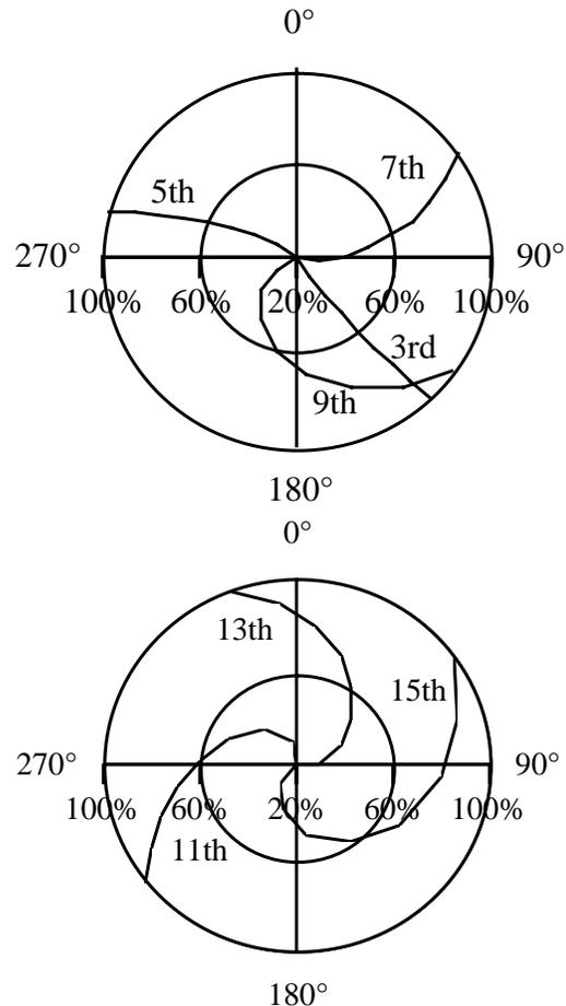
Figure 3. Harmonic Current Phase Angle Variation Versus Load Power for Heat Pump Example
