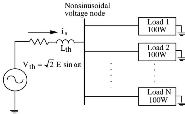
Figure 4. N Identical Computers Served by a 120 V Branch Circuit
