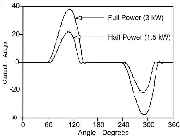
Figure 2. ASD Current Waveforms for 50% and 100% Power
