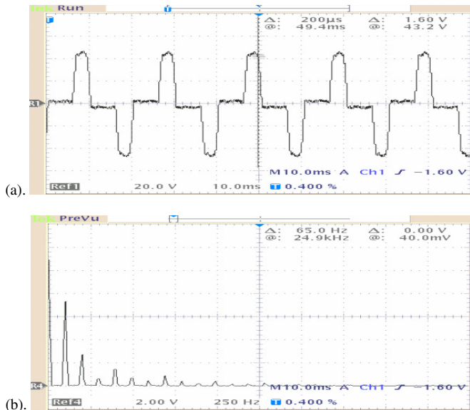
Fig. 1. (a). Recorded current waveform and (b). Harmonic spectrum for PC load current.
