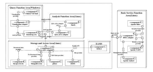
Fig. 4. The UML deployment diagram presents the main components, communication channels and technological requirements of four areas.
