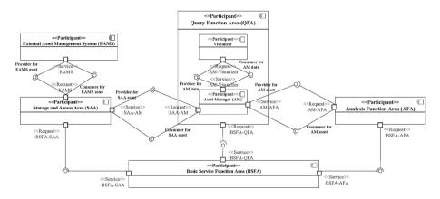
Fig. 2. Software architecture diagram shows the internal composition of each area and interaction with other areas through interfaces.
