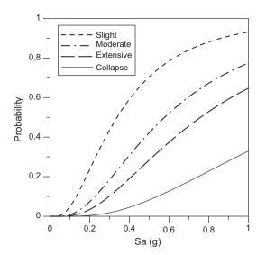
Fig. 13. Fragility curves of the 12-story Type B model structure without vierendeel panels.
