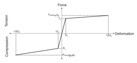
Fig. 22. Idealized backbone curve of the BRB.
