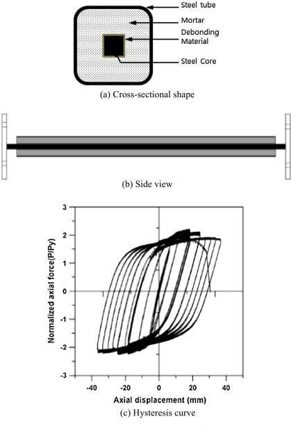
Fig. 21. Buckling restrained brace used in the retrofit design.
