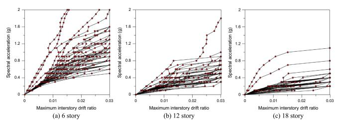
Fig. 10. Incremental dynamic analysis results of the structures with 2 m-wide middle corridor.
