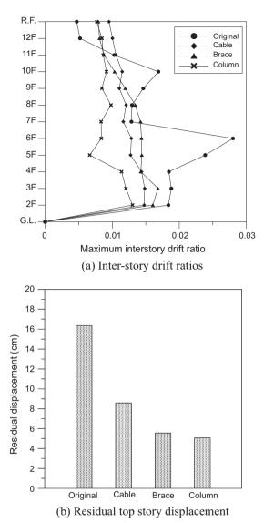
Fig. 18. Mean responses of the 12-story Type A structures subjected to strong earthquakes.
