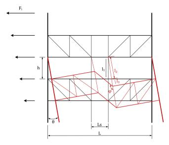
Fig. 15. Deformed configuration of a Type A structure reinforced with cables.
