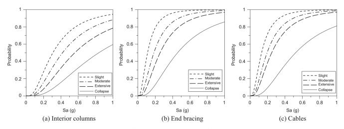
Fig. 19. Fragility curves of the 12-story Type A structures retrofitted with various methods.
