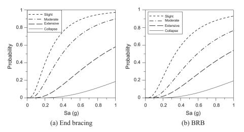
Fig. 25. Fragility curves of the retrofitted Type B structures.
