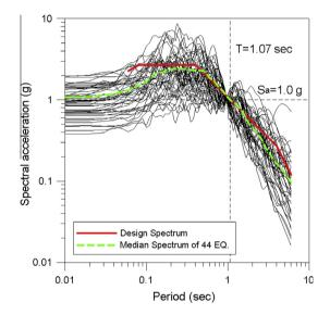
Fig. 9. Response spectra of the 44 scaled ground motions scaled to the fundamental period of 1.07 s.
