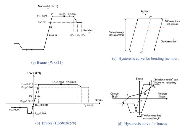
Fig. 4. Nonlinear force-displacement relationship of structural members.
