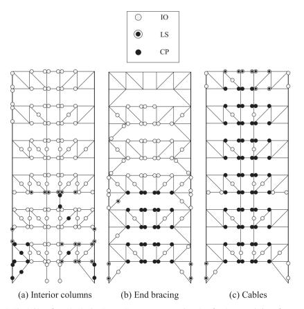
Fig. 17. Plastic hinge formation in the 12-story Type A structure at the point of major strength drop after retrofit.
