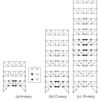
Fig. 7. Plastic hinge formation in the Type A structures.
