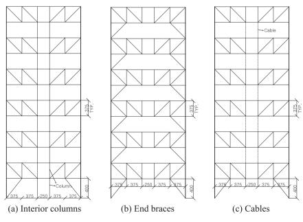
Fig. 14. Seismic reinforcing schemes for Type A structures.
