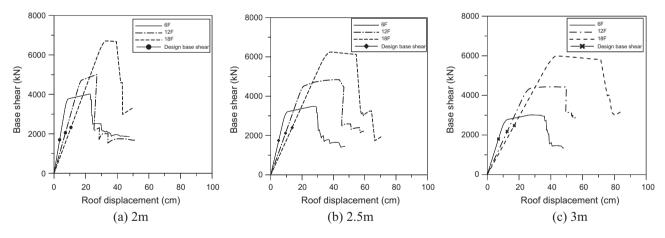
Fig. 5. Pushover curves of Type A STS model structures having vierendeel panels with different lengths.
