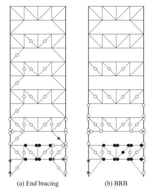
Fig. 24. Plastic hinge formation of the Type B structures after retrofit.
