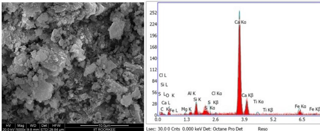
Fig. 7. SEM-EDX Micrographs of CM specimen at 28 Days.
