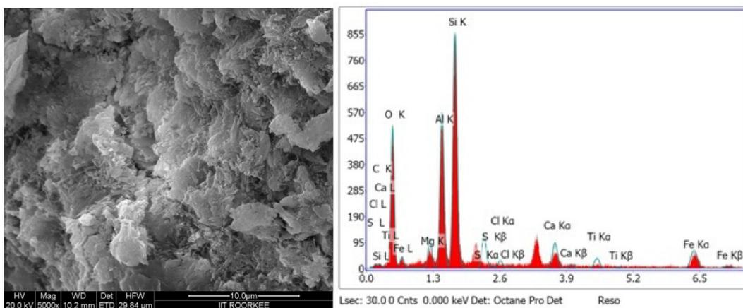
Fig. 10. SEM-EDX Micrographs of MN2 specimen at 28 Days.
