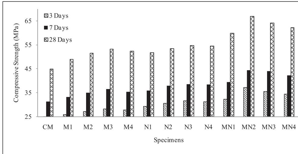
Fig. 4. Compressive Strength of Specimens at 3, 7 and 28 Days.
