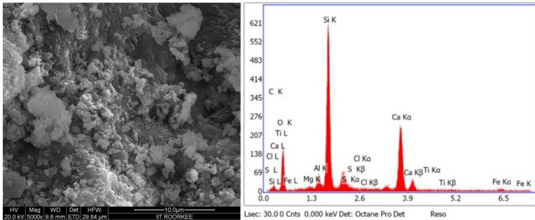
Fig. 8. SEM-EDX Micrographs of M3 specimen at 28 Days.
