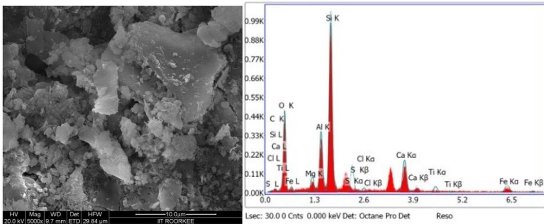
Fig. 9. SEM-EDX Micrographs of N3 specimen at 28 Days.
