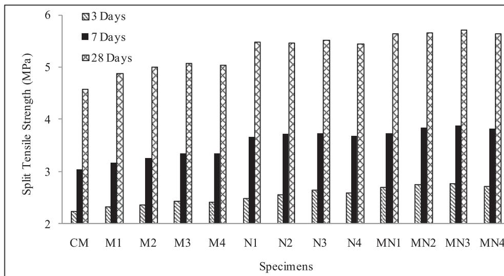
Fig. 5. Split Tensile Strength of Specimens at 3, 7 and 28 Days.
