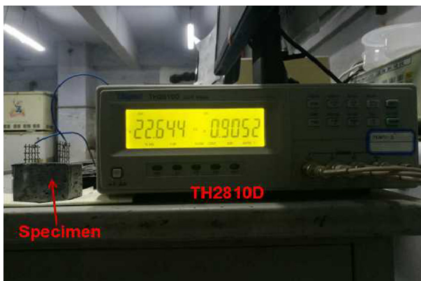
Fig. 2. Electrical resistance measurement.
