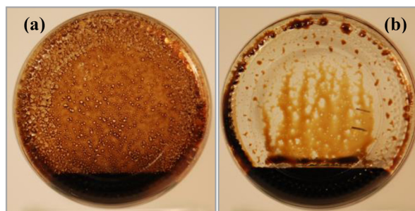
Figure 8—Crude oil sample mixed with different solvents at 25°C – (a) Xylene and (b) solvent/co-solvent mixture.
