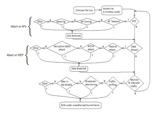
Fig. 3. Wireless Network Attack Tree.
