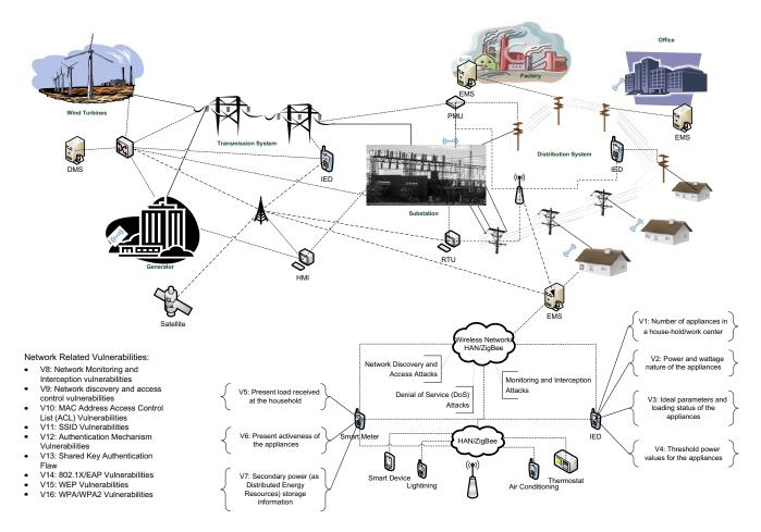
Fig. 2. SG Block Diagram with Communication Network and Devices.
