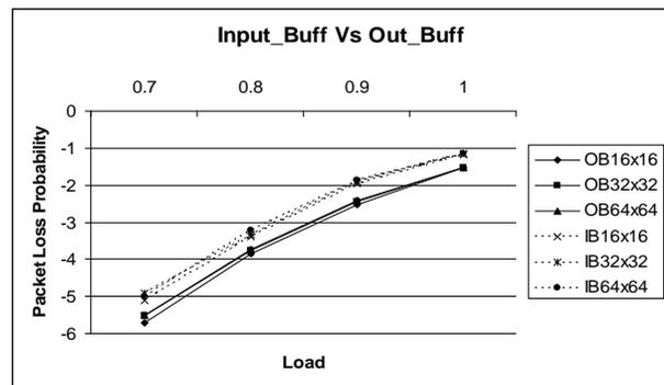
Figure 10. Comparing packet loss probabilities for input buffered and output buffered architectures for different switch sizes.
