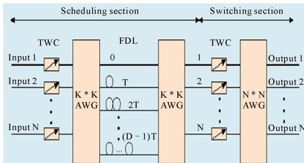
**Figure 6.** Input buffered optical packet switch.
